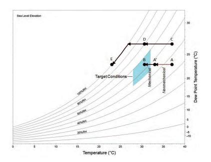
Figure 5.10 Implementation of mechanical cooling.
