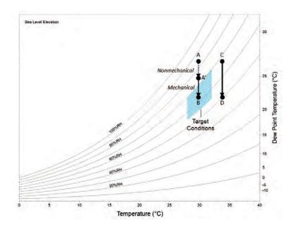
Figure 5.7 Implementation of mechanical dehumidification.
