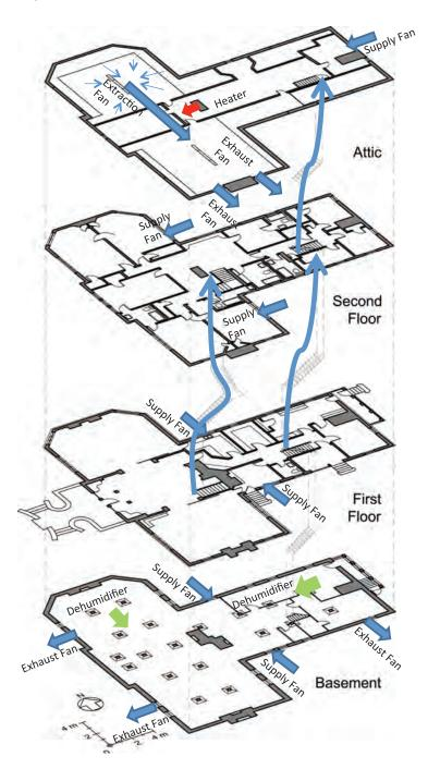
Figure 10.2 Locations of mechanical system components during the case study, part B.
