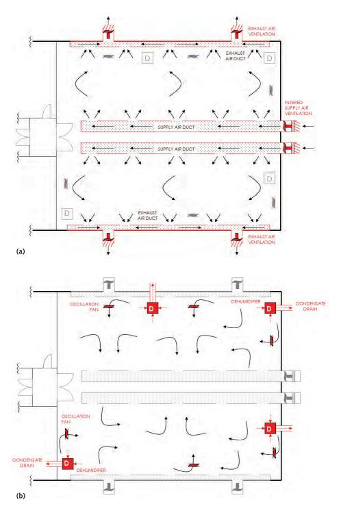
Schematics of the psychrometric modes of operation for the environmental management system at the Goeldi Museum's new storage facility: conservation heating by ventilation (a) and dehumidification (b).
