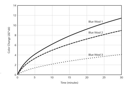
rapid for a relatively new object, the eventual loss of reaction sites could slow the rate of chemical damage over time. This shift in chemical reactivity is shown graphically in figure 2.9, where the rate of light-induced chemical color change declines following an initial period of rapid color change.
