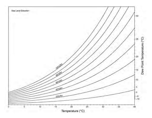
Figure 5.1 Psychrometric chart for sea level elevation.
