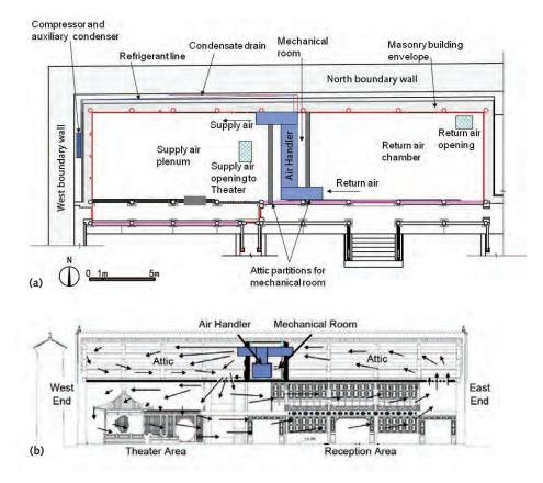
Attic floor plan showing the mechanical room and the locations of environmental management system components (a), and the airflow of conditioned air in the building (b). Schematic (b): Shin Maekawa. © J. Paul Getty Trust.
