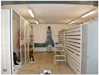
Side panels of the compact shelving system are made of perforated sheet metal to allow airflow through the panels even when the shelving units are closed (a); the fronts of the steel drawer cabinets have gaps to permit air circulation even when the drawers are closed (b). Photos: Shin Maekawa. © J. Paul Getty Trust.
