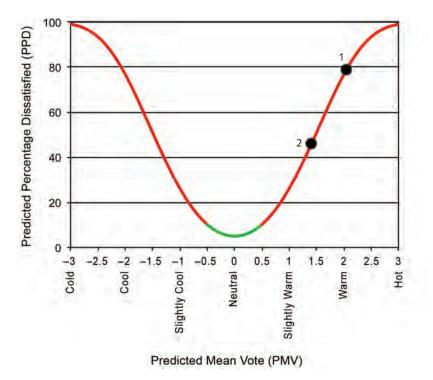
PMV-PPD plot showing thermal comfort in the storage room during the dominant rainfall season with an air speed of 0.5 m/s (1), and an air speed of 3 m/s (2).
