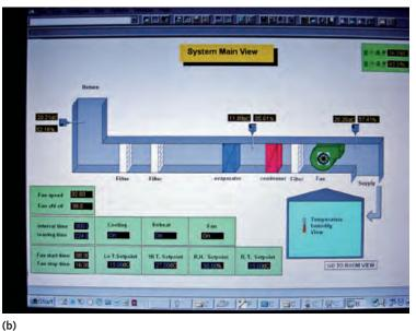
Operation of the environmental management system can be monitored with a keypad and display unit installed in Juanqinzhai (a) or via an office PC that connects remotely to the system through the Palace Museum's LAN (b).
