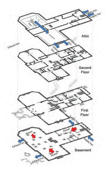
Figure 9.11 Locations of mechanical components in the basement and attic.
