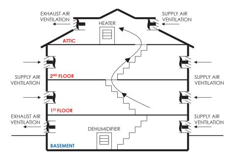
**Figure 10.1** Schematic of whole-house ventilation/ basement dehumidification/attic heating.
