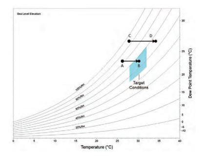
Figure 5.8 Implementation of mechanical heating.
