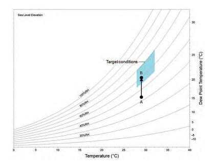
Figure 5.11 Implementation of mechanical humidification.
