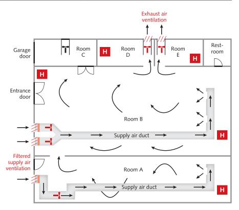
**Figure 12.12** Schematic of conservation heating by ventilation mode.
