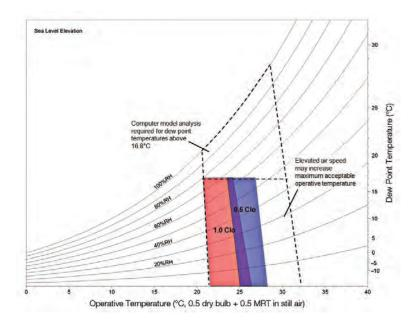
environments with dew point temperatures above 16.8°C, as is common in hot and humid climates. As discussed in chapter 4, the use of elevated air speeds can also provide a cooling effect for occupants and will expand the thermal comfort zone by allowing for higher acceptable maximum operative temperatures (defined as: ½ dry bulb temperature + ½ mean radiant temperature).
