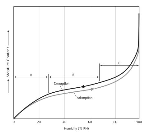
**Figure 2.3** Adsorption and desorption isotherms for a generic hygroscopic material.
