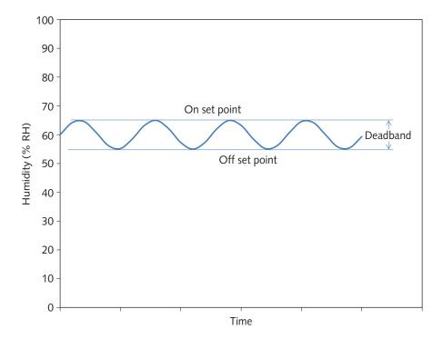
Figure 7.14 Schematic of set points and deadband.
