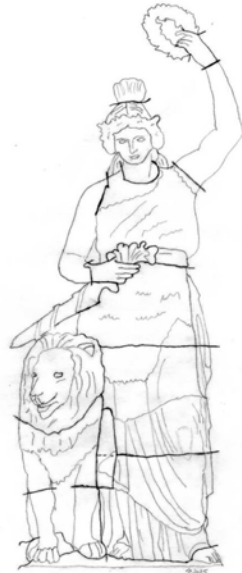
Figure 2.6. Statue of Bavaria. The edges of the large cast pieces are marked Image: © Ursula Vedder
