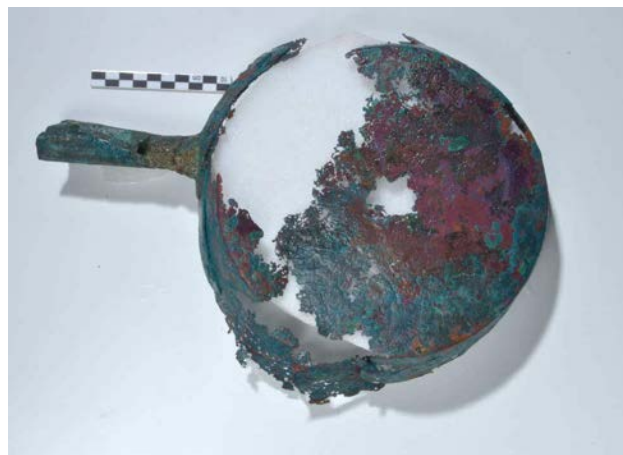
Figure 38.8a. The frying pan before treatment with local electrolysis and the corrosion inhibitor L-cysteine
