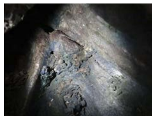
Figure 41.2. Bronze spillage and azurite buildup on herm boss and head interior
