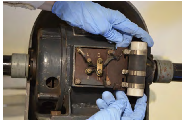
Figure 16.1. Detail of one of the inner dynamos in the Cockcroft-Walton generator.
