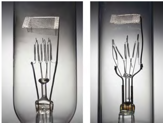
Figure 4.7. Manufactured and handmade 1,000W tungsten filaments.
