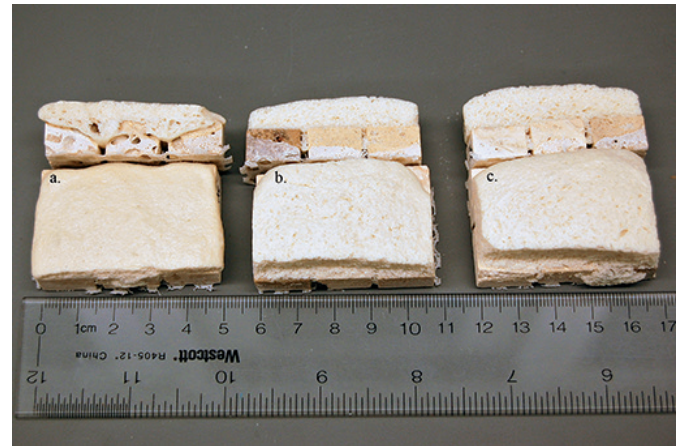
Figure 4 The effect of increasing the amount of Rencast 1774 foaming agent on the foaming of the Rencast 1774 epoxy system (all formulations include 10 g Rencast 1774 resin, 2.5 g Rencast 1774 hardener, and 0.3 g Cabosil TS720 as well). (a) 0.12 g foaming agent; (b) 0.38 g foaming agent; (c) 0.50 g foaming agent. Credit: Institute for the Preservation of Cultural Heritage, Yale University
