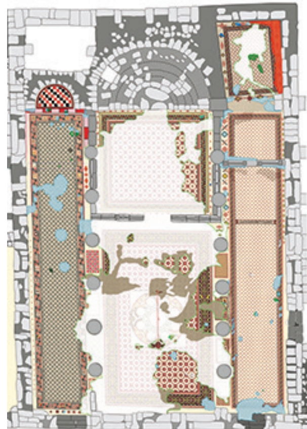
Figure 2 Condition and treatment mapping of the mosaic floor in the North-West Church in Hippos-Sussita executed in metigoMAP graphic software.
