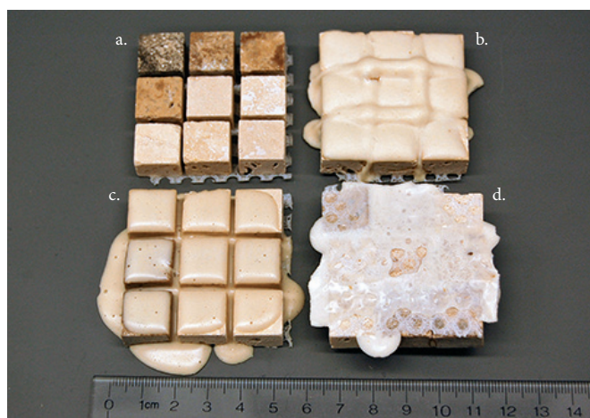
Figure 3 Properties of the Rencast 1774 (Rencast) epoxy system mixed and poured according to the manufacturer's guidelines. (a) Uncoated 3 × 3 tiles, adhered on the bottom with a mesh, used as a mock-up. (b) 10g Rencast resin (R):2.5 g Rencast hardener (H):0.125g Rencast foaming agent (A). (c) 10g R:2.5g H:no foaming agent. (d) Back side of the 3 × 3 tiles showing how the 10g R:2.5g H:0.125g A mixture flowed through the gaps between tiles and covered the back. Credit: Institute for the Preservation of Cultural Heritage, Yale University
