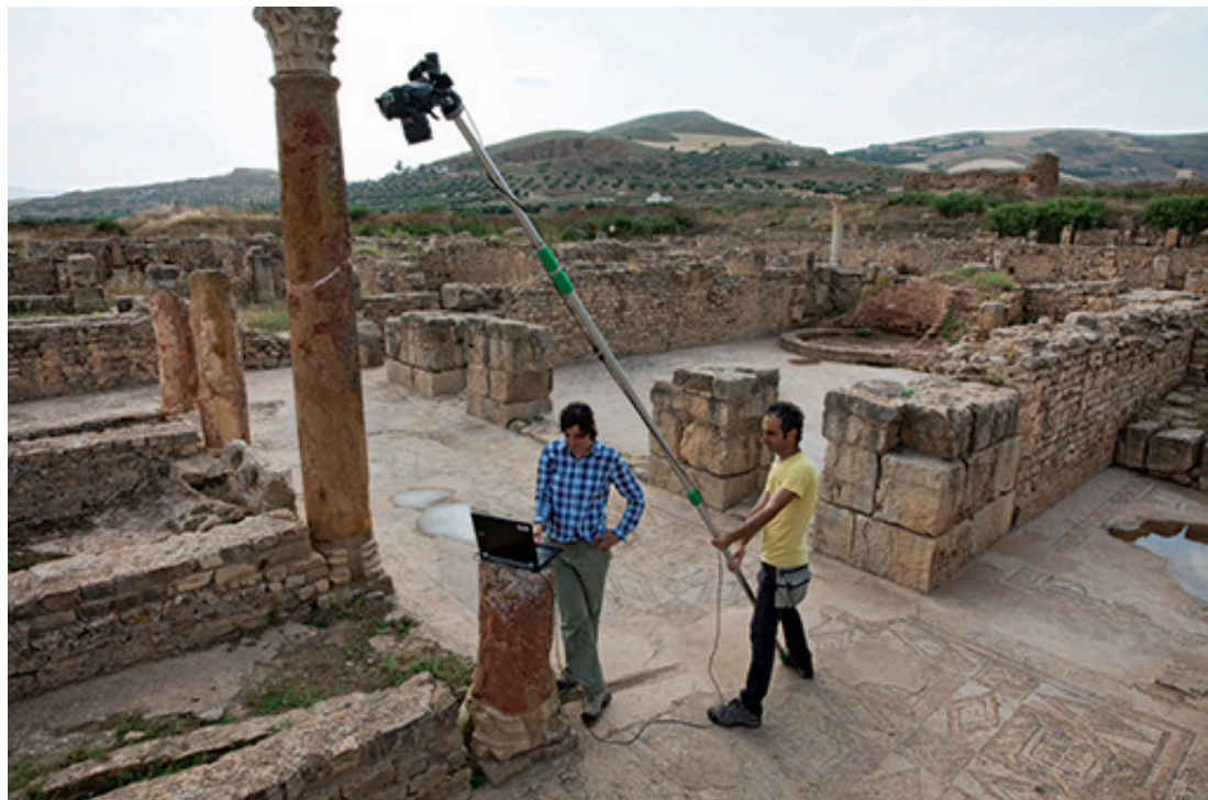
Figure 1 Photographic survey of site mosaics using a lightweight extension pole.
