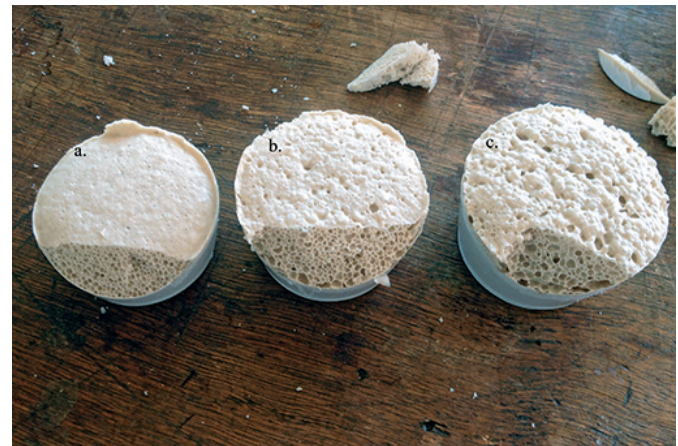
Figure 6 Effect of foaming agent on the Hodgson foams made with 10% Epon 828, 20% diluent, and 70% English whiting. (a) 1 vol. % foaming agent (FA); (b) 2 vol. % FA; (c) 3 vol. % FA. Credit: RH Conservation Engineering
