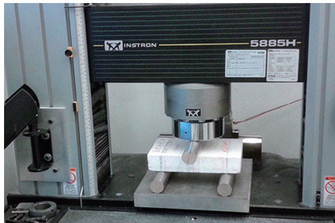
Figure 3 Flexural-tensile strength testing on a mid-scale mockup placed into an in-house built testing fixture loaded by the Instron Universal Testing Machine.
