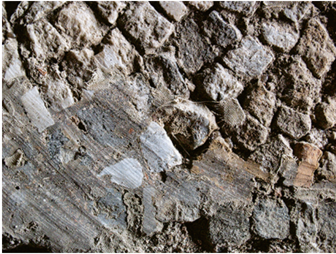
Figure 3 Previously restored mosaic fragment damaged by migration of epoxy to the mosaic surface and facings. Evidence of rough scratching of the epoxy and facing material, thus causing additional deterioration of the tessellatum. Photo: Elena Kantareva-Decheva, 2011
