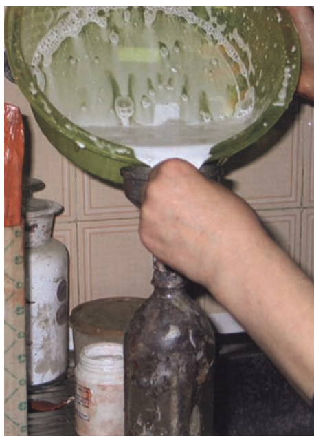
FIGURE 5 (A) Vulcano V7 PVA emulsion mixed with water; (B) paint prepared with V7 and red ochre (both prepared by Sofia Agrela).
