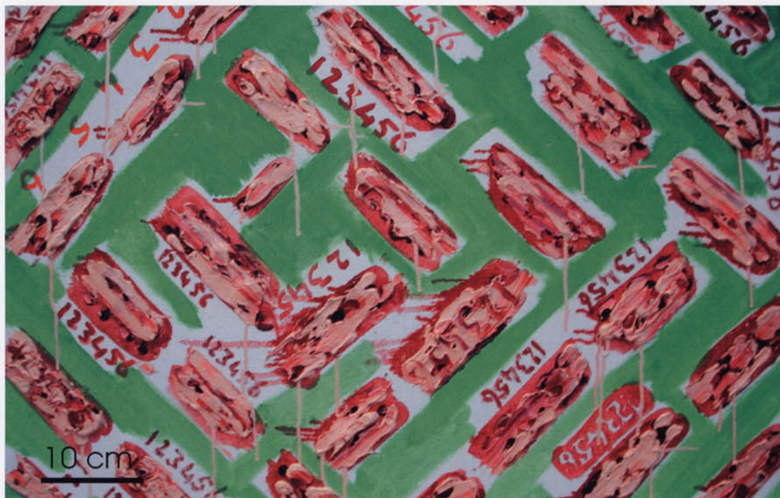
FIGURE 1 A painting by F. van H. shows disturbing paint defects of melting impasto and vertical flesh-colored drips caused by physical separation of paint components after an initial drying period of six years. Published with permission of the artist.
