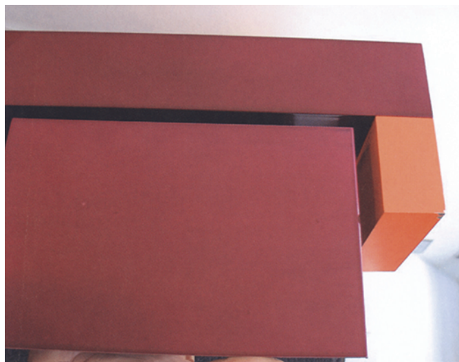
FIGURE 7 Side-by-side comparison of paint applied to a test panel and the Phoenix sculpture, showing a very good color match. Photo: Eleonora Nagy.
