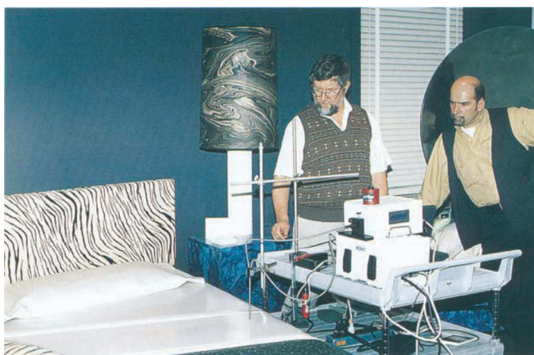
FIGURE 2 Portable infrared spectrometer used in situ in the identification of plastics.
