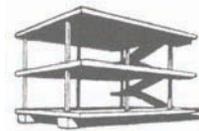
Fig. 87. **LE CORBUSIER.** Ferroconcrete Skeleton Frame for the Housing Settlement "Domino" 1915
