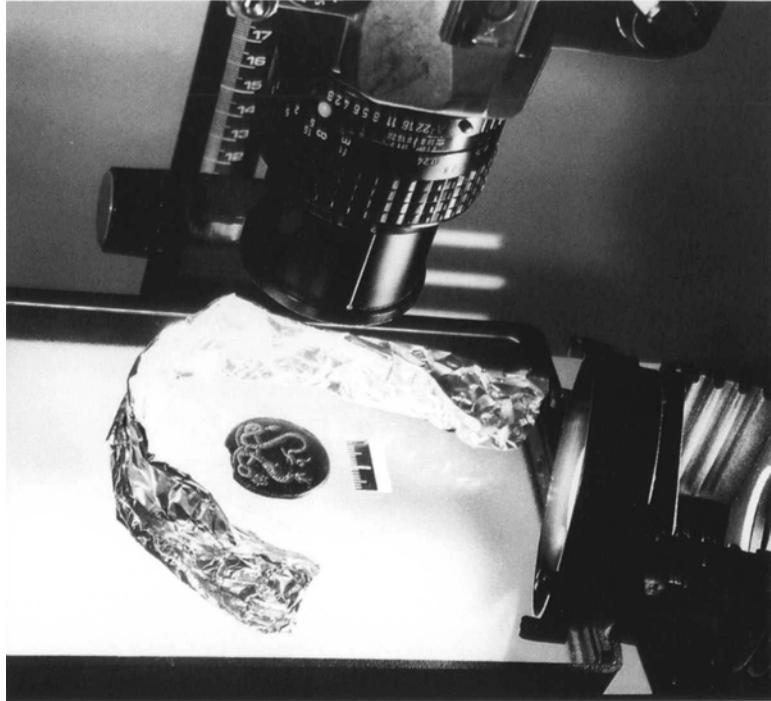
Figure 23 **A reflective low wall of crushed and reflattened aluminum foil used to bounce light into shadows produced by the light source.**
