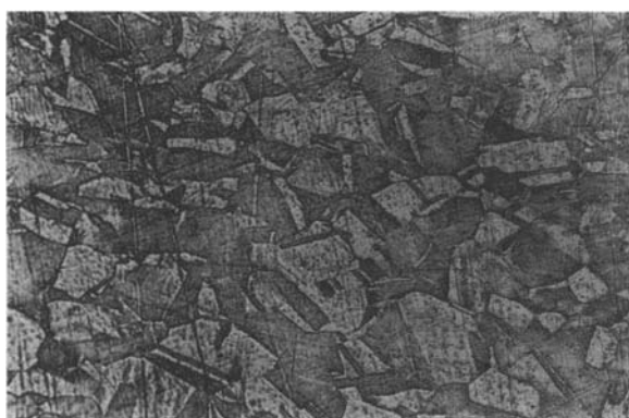
Fig. 17. Etched metallographic section of Erimi hook no. 7, mentioned in Dikaios' day book and found in the Nicosia Museum by D. Bolger among the Erimi material (Photomicrograph by N. H. Gale).
