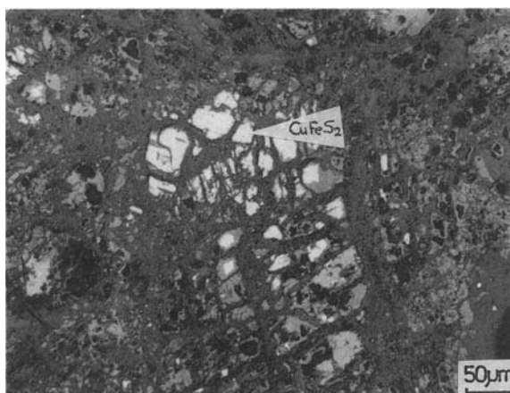
Fig. 12. Polished section of another area of KM 633, showing the presence of the copper ore chalcopyrite, \text{CuFeS}_2 (photomicrograph by U. Zwicker).
