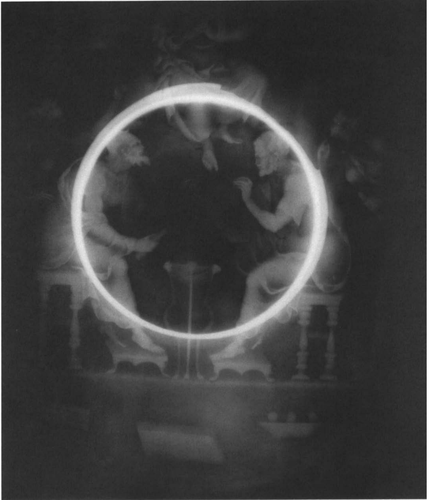
Figure 3. Print made from an X-radiograph of the Philosophers plate taken at 250KV, 8mA for 2.5 minutes at a distance from source of 50 inches. The figurative detail shows strong contrast due to the thicker silver in these regions compared with the background. The radiograph does not help to answer the question of how the footring was attached, no solder or join being evident.
