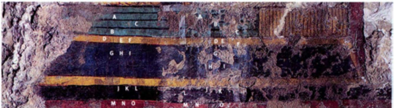
Because of inhomogeneity in the colors of the wall paintings, and the difficulty in precisely locating the measuring head at each desired point, three locations within each colored area were selected for measurement, and each location was measured three times. Instrumental reproducibility was calculated from the replicate measurement data.
