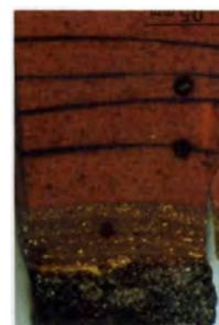
Figure 24. Part of the cross section of No. 15 (Fig. 23), showing the yellow ground layers (x63).
