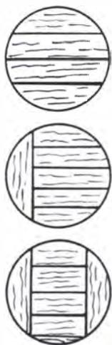
Figure 1 a-c. Construction of central base.
