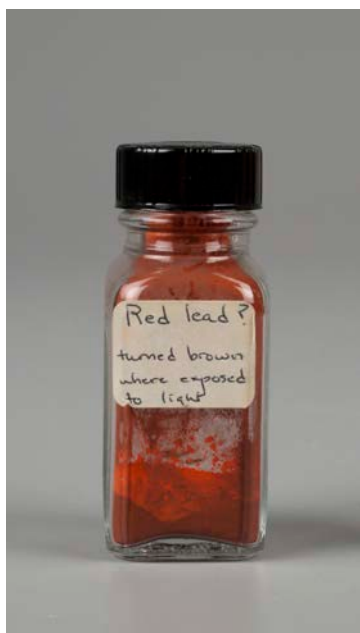
Figure 17.13 Jar of red lead from the Forbes Pigment Collection showing darkening caused by light exposure. Harvard Art Museums/Straus Center for Conservation and Technical Studies, Forbes Pigment Collection, Straus, 1707. Photo: © President and Fellows of Harvard College
