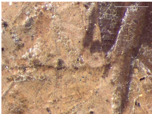
Figure 14.5 Photomicrograph showing blue particles visible in the paint surface of the highlight under the sitter's right eye, corresponding to the regions with VIL responses for Egyptian blue (fig. 14.2) and XRF responses for copper (fig. 14.3A), as seen in the stereobinocular microscope with fiber optic illumination. Photo: S. Spence, Courtesy of the Nelson-Atkins Museum of Art
