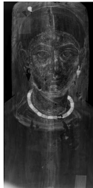
Figure 14.4 X-radiograph revealing greater radio-opacity associated with the M-shaped lines of Egyptian blue seen in the VIL image (fig. 14.2) and the greater thicknesses of the relief decorations, including those visible in the Cu distribution map (fig. 14.3A). Settings: 60kV; 3mA; 5 second exposure; film. Photo: J. Rogers, Courtesy of the Nelson-Atkins Museum of Art
