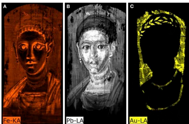
Figure 12.16 Portrait of a young woman with a gilded wreath (Portrait G), elemental distribution maps obtained by MA-XRF: (A) iron (Fe), (B) lead (Pb), and (C) gold (Au). Photos: © The Metropolitan Museum of Art, Department of Scientific Research
