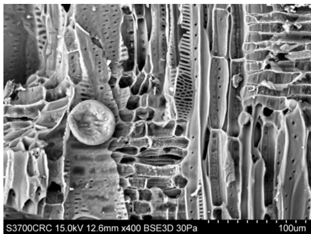
Figure 6.6 Scanning electron microscope image of a radial longitudinal section of Fagus sylvatica (European beech) wood from CA 5878 (ST). It shows (among other features) scalariform and reticulate perforation plates, one tylosis (of many), and rays with procumbent cells and square marginal cells. The condition of this wood is similar to modern fresh wood samples; it is unlike the condition of other mummy portrait woods. The presence of scalariform and reticulate perforation plates shows clearly that it is beech rather than oak, which has simple perforation plates. Photo: C. R. Cartwright. © The Trustees of the British Museum
