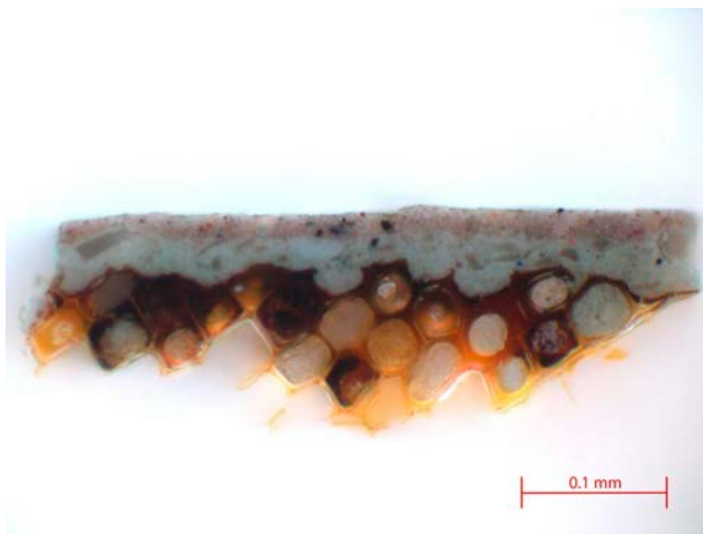
Figure 6.3 Cross section taken from the gray background of 1970-001 DJ (ST) (fig. 6.1), showing a portion of the wooden substrate, the greenish ground that contains the modern pigments barium sulfate and Prussian blue, and the surface gray paint. Photo: C. E. Rogge
