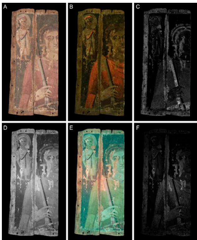
Figure 3.5 Multiband imaging of panel ÆIN 685: (A) VIS, (B) UVF, (C) MBR, (D) IRR, (E) FCIR, (F) VIL with a small contribution from IRR. Photo: Jens Stenger
