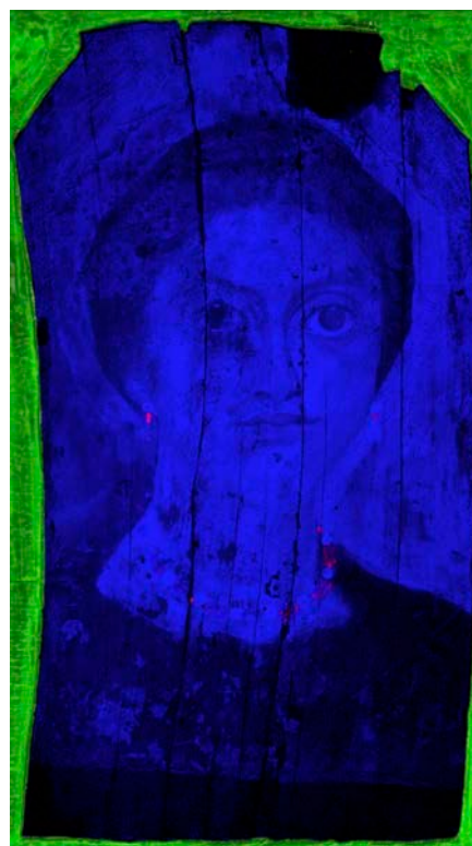
Figure 1.7 False-color MA-XRF map of the Lady showing the signals for As-K (red), Ti-K (green), and Pb-M (blue). Acquisition and processing of the MA-XRF maps by Erma Hermens, Annelies van Loon, Victor Gonzalez, and Francesca Gabrieli. Photo: False-color imaging by Jan van Daal
