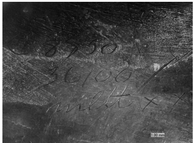
Fig. 1.16 Photomicrograph of a lightly scribed notation on the underside of vessel foot (82.DG.17.b), to the right of the more heavily inscribed “384 14” [crossed out]. Image captured at 20x magnification with a Keyence digital microscope. Image: Karen Bishop
