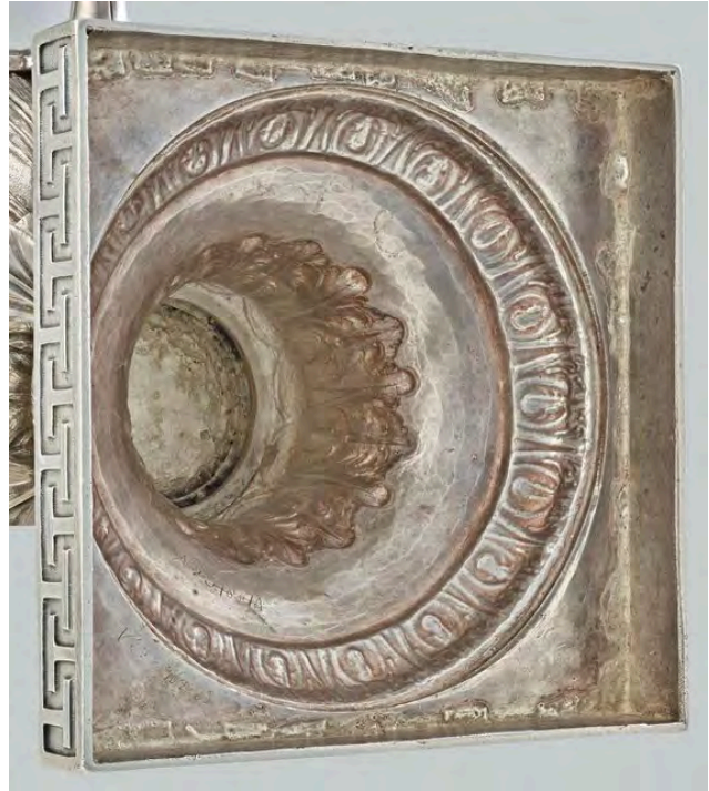
Fig. 1.15 Underside of body, foot, and base of vessel (82.DG.17.b) revealing large pallions of solder along the top of the square base. The top sheet of the base has a round cutout of the center, which has been soldered to the foot.
