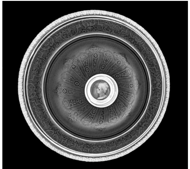
Cat. 2.3 Lid (71.DG.77.a), X-radiograph showing the female profile that may have been separately cast and soldered on the spool-shaped knob.
