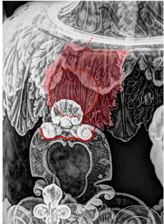
Fig. 1.13 X-radiograph of vessel (82.DG.17.b) showing the interior and exterior repair patch. Red highlighting indicates exterior patch material, the solid red line emphasizes the fine exterior separation, and dotted red lines represent seams visible on the interior.
