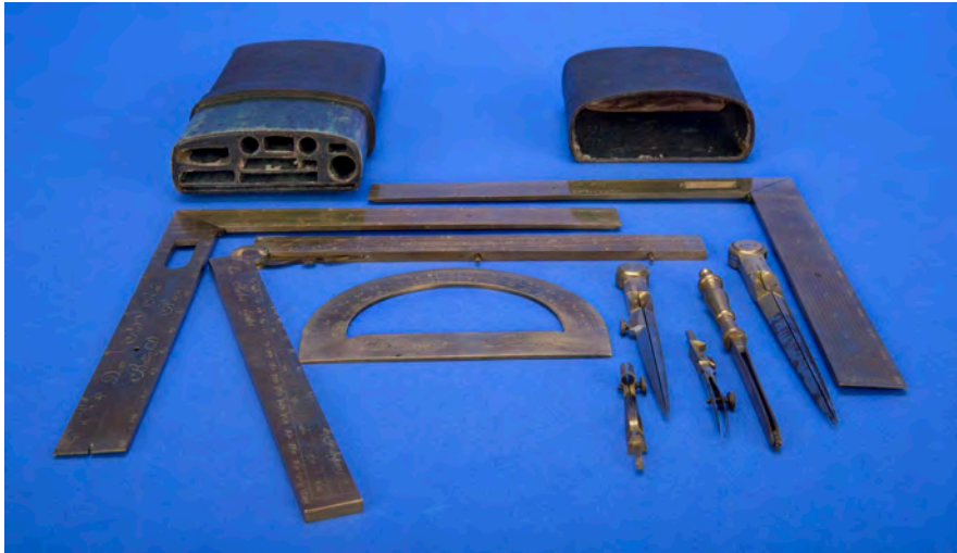
FIG. 134 Michael Butterfield, Porte-crayon and other drawing instruments with their case, ca. 1700. Brass instruments and leather case. Washington, Division of Medicine and Science, National Museum of American History, Smithsonian Institution.
