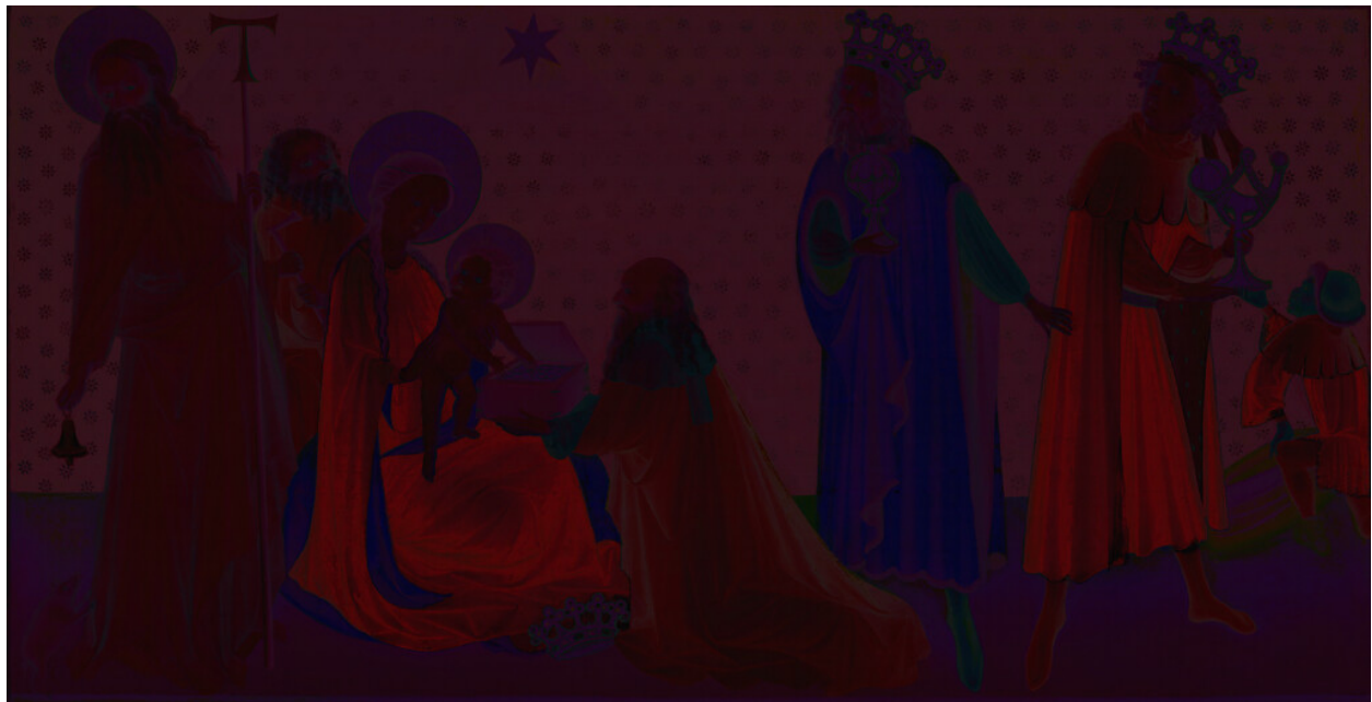
Quantitative difference (brighter areas are more different) between original and JP2 derivative.
