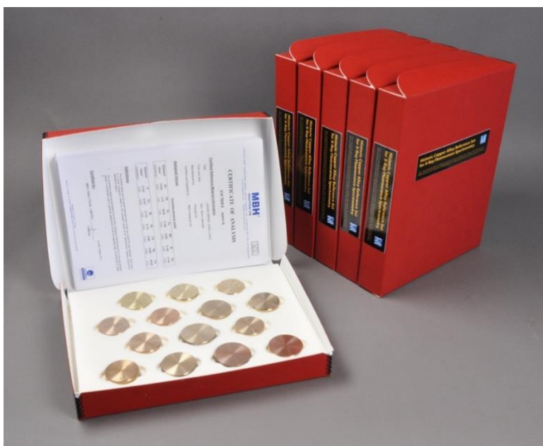
The first Copper Cultural Heritage Alloy Reference Material (CHARM) Sets; each set pictured contains the core set of twelve certified reference materials (CRMs) plus two supplementary high-arsenic CRMs.
