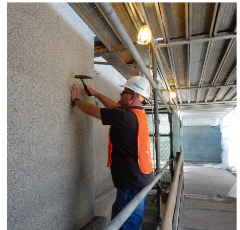
Figure 3. CTL Group conducting a condition assessment of the existing shotcrete.
