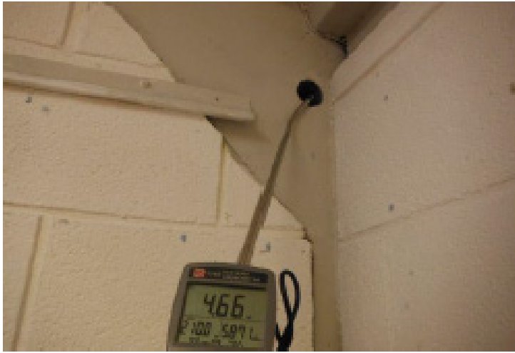
7. Wall Plate Some of the wall plate to roof junctions showed leakages; here is a reading from F4 showing a leak of 3.11m/s.
