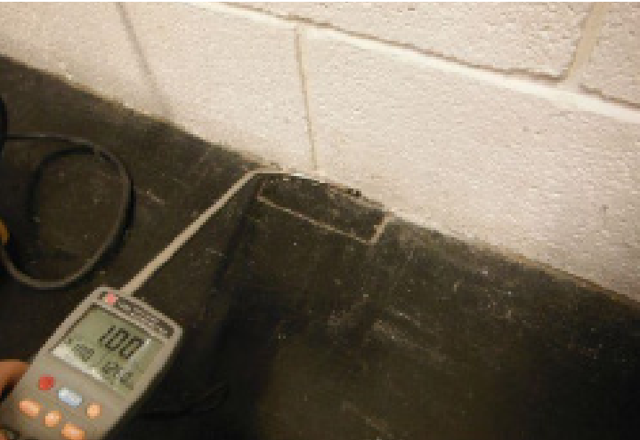
5. External Door The exit door at D4 has considerable air leakage problems. Shown here is a reading at the head of the door showing 4.85m/s air leakage.
