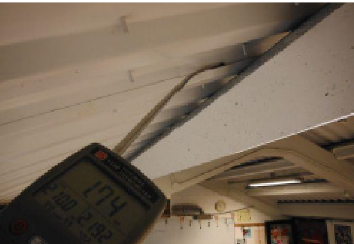
10. Roof Panels Generally the roof was well sealed but some air leakage was detected in each room, here shown in F4 at 1.74m/s.
