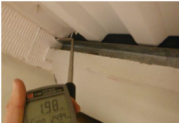
9. Fireseal Small gaps were identified in this seal, here shown in F1 reading 1.98 m/s.
