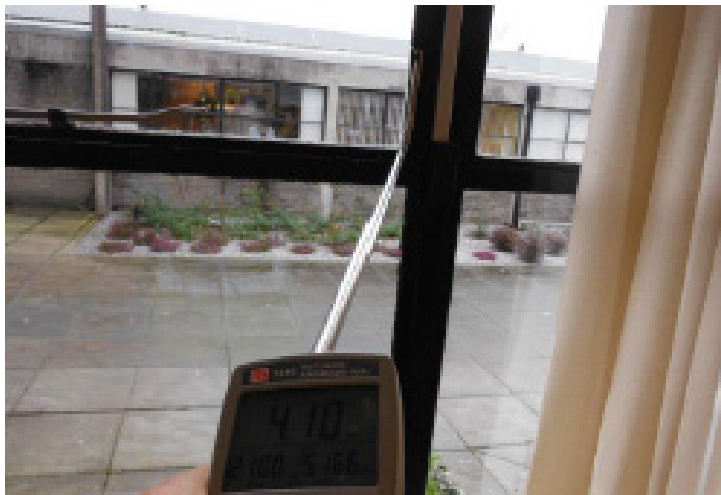
9. Fireseal Small gaps were identified in this seal, here shown in F1 reading 1.98 m/s.
