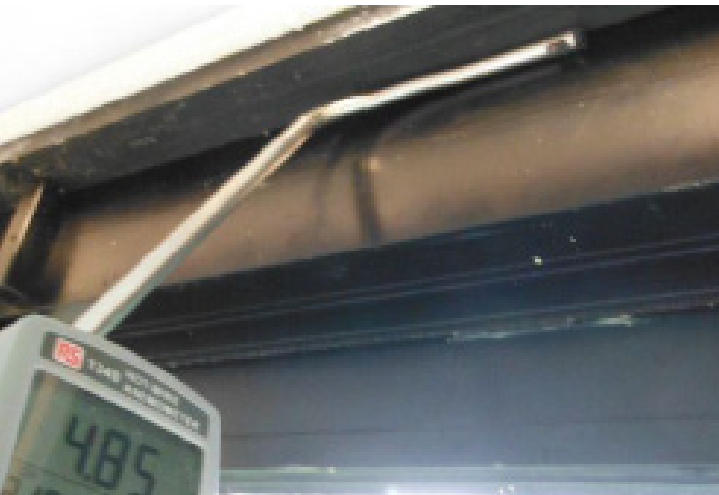
10. Roof Panels Generally the roof was well sealed but some air leakage was detected in each room, here shown in F4 at 1.74m/s.
