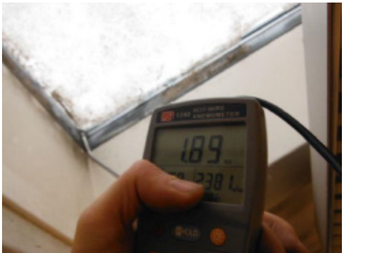
11. Rooflight Generally these were well sealed, though some air leakage was identified, below shown in F1 at 1.89m/s.
