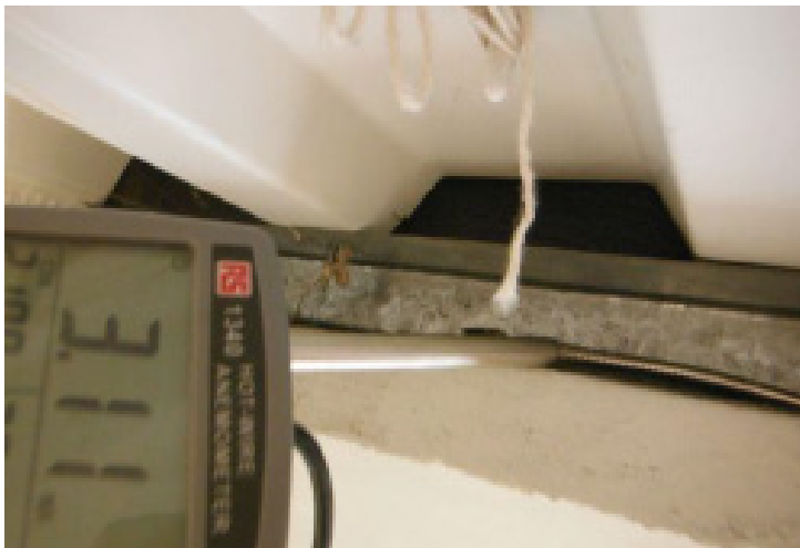
11. Rooflight Generally these were well sealed, though some air leakage was identified, below shown in F1 at 1.89m/s.
