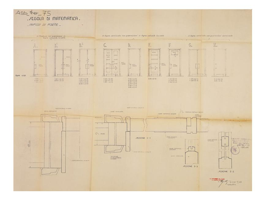
Figure 15 - The doors supplied by the firm Cantieri Milanesi; the drawing specifies models, materials and finishing processes (ASS\_drw\_75)
