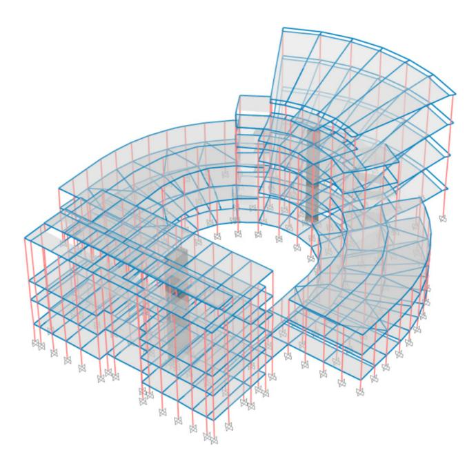
Figure 40 - 3D model of the building in its original configuration in 1935 (© Martella 2020) nal forces (axial and shear forces, bending moment) used for the element sections design, i.e. to design the reinforcement. Modal analysis was carried out to evaluate the vibration modes and period of vibrations of the structure with the aim to compare such characteristics with those obtained for the building in its current configuration.
