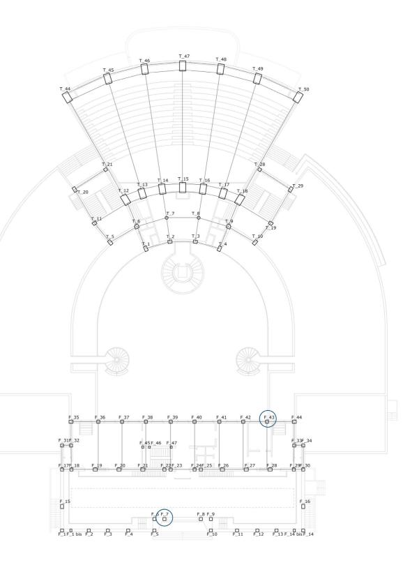
Figure 11 - Structural elements identification numbers and location of the rebar locating tests, third level (© Martella 2020)
