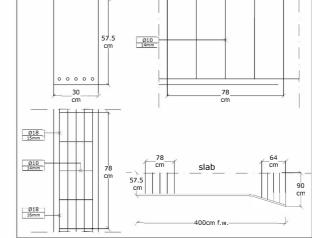
Figures 12/15 - Rebar locating tests data sheets (© Martella 2020)
