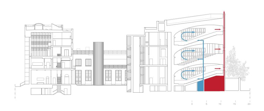
Figure 24 a/b - Diagram of hot air circulation system in the tiered lecture halls: blue arrows indicate the delivery section of air, red expulsion (© Mancini 2020), and an image of the tower of the 1930s where the chimney is still visible (ASS\_pht\_05)
