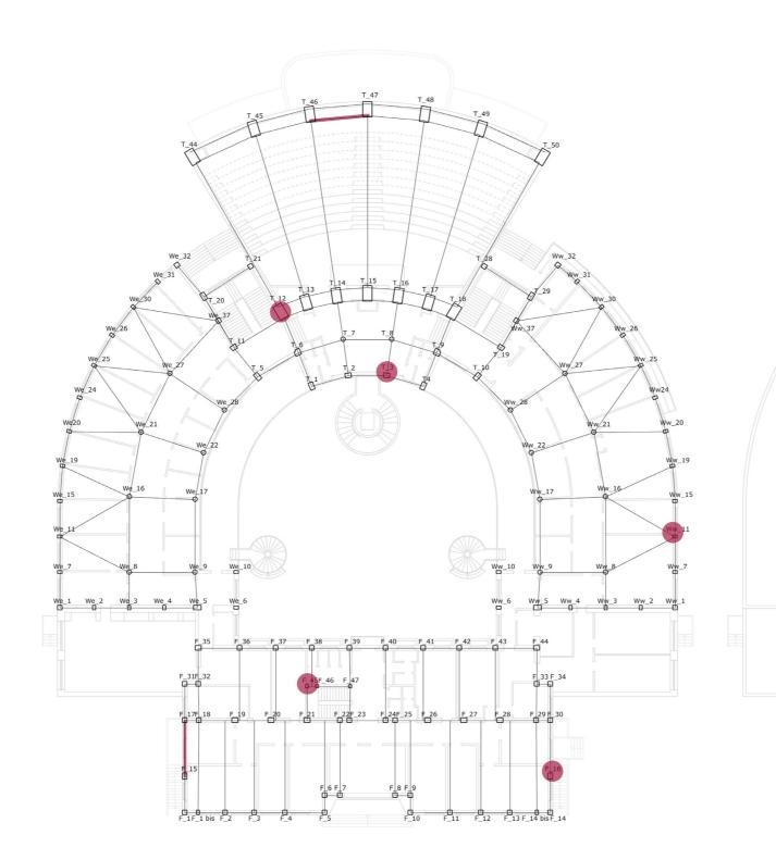
Figure 47 - Not satisfactory structural elements: first level (© Martella 2020)
