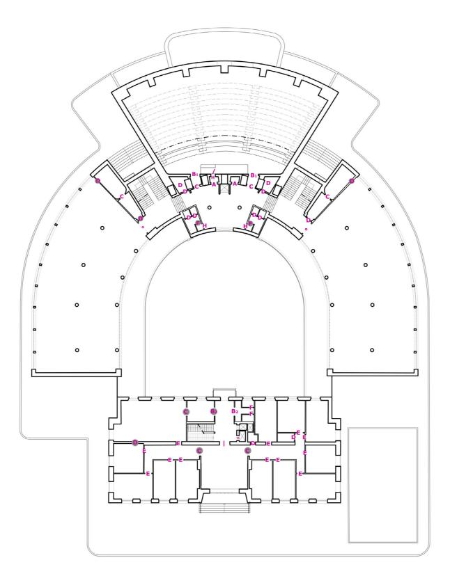
Figure 9 - Mapping of doors in 1935 and 2021, at the first level (© Bardati, Turco 2021)
