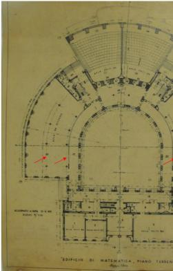
Figure 10 - Plan of the ground level as of December 18, 1933 (ASS\_drw\_25). Columns highlighted with red circles are not present in a drawing dated 1935 as well as in the building
