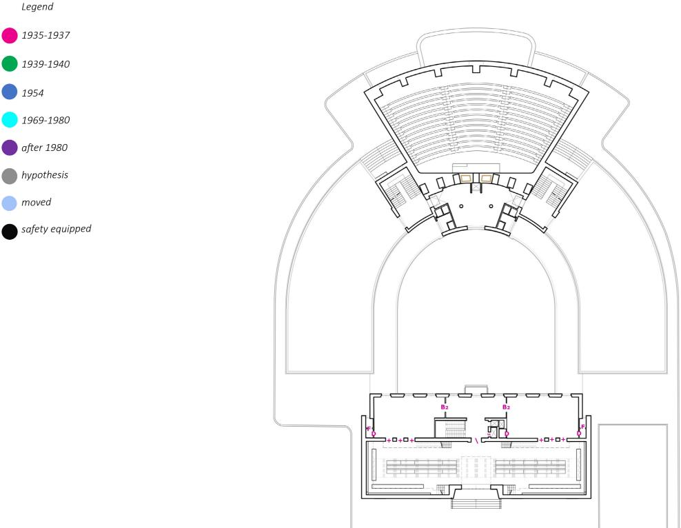
Figure 10 - Mapping of doors in 1935 and 2021, at the second level (© Bardati, Turco 2021)
