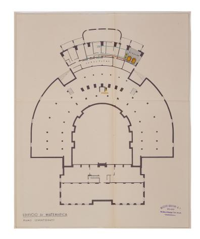
Figure 1 - "Basement plan" of the Mathematics building indicating the intersection between the independent and centralized heating plant, 1942 (ASS\_ drw\_131)
