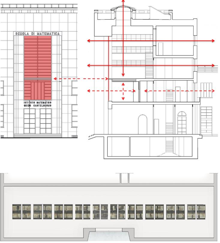
Figure 10 - Visual and spatial axes of the front building destroyed by the addition of horizontal elements, partitions, and the canopy over the skylight (© Salvo 2012)
