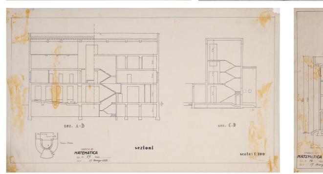
Figure 14 - "Tower Façade" of the Mathematics building, March 17 1933; actually, this is a cross section along the side entrances (ASS\_drw\_16)
