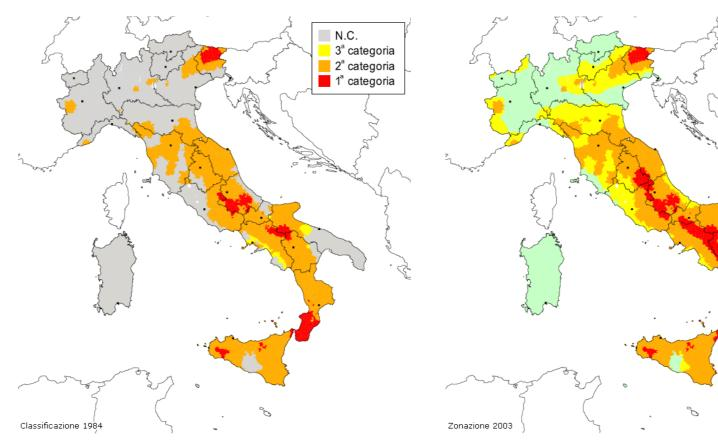
Figure 36 - Seismic classification in 1984 (BBL\_drw\_17)
