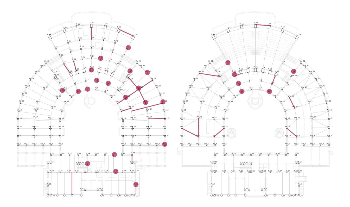
Figure 45 - Not satisfactory structural elements: basement level (© Martella 2020)
