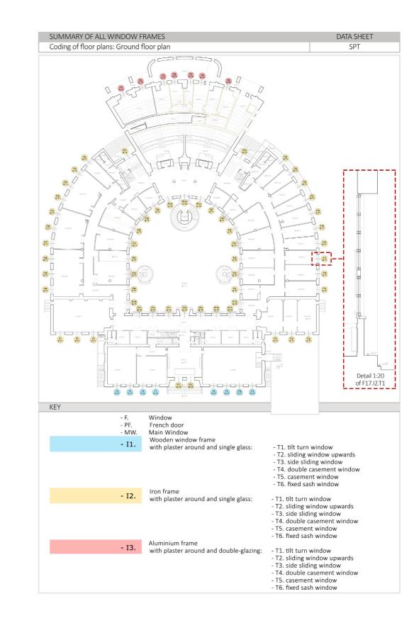
Figure 30 - Sample of window mapping at the ground floor, with detail of one type of window (© Romano 2020)
