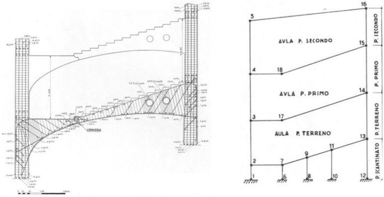
Figure 19 - Schematic representation of the beams at the intermediate levels of the tower of classrooms
