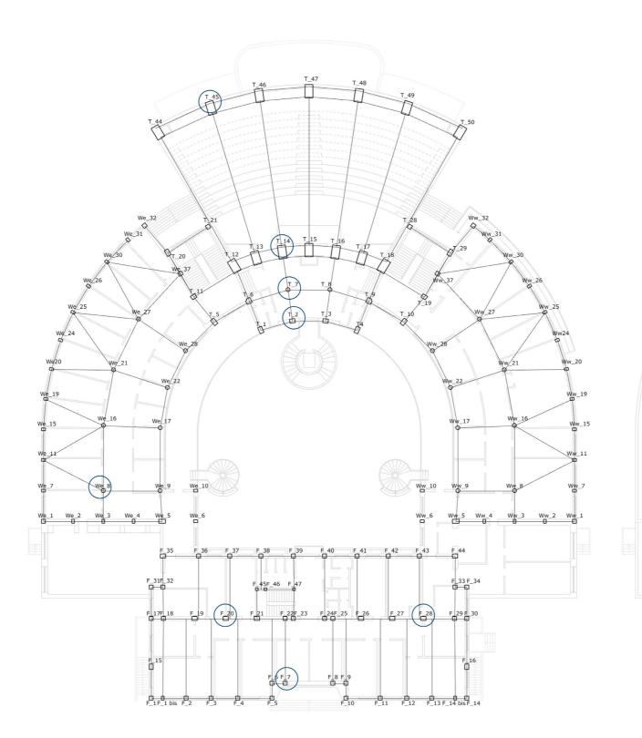
Figure 9 - Structural elements identification numbers and location of the rebar locating tests, first level (© Martella 2020)
