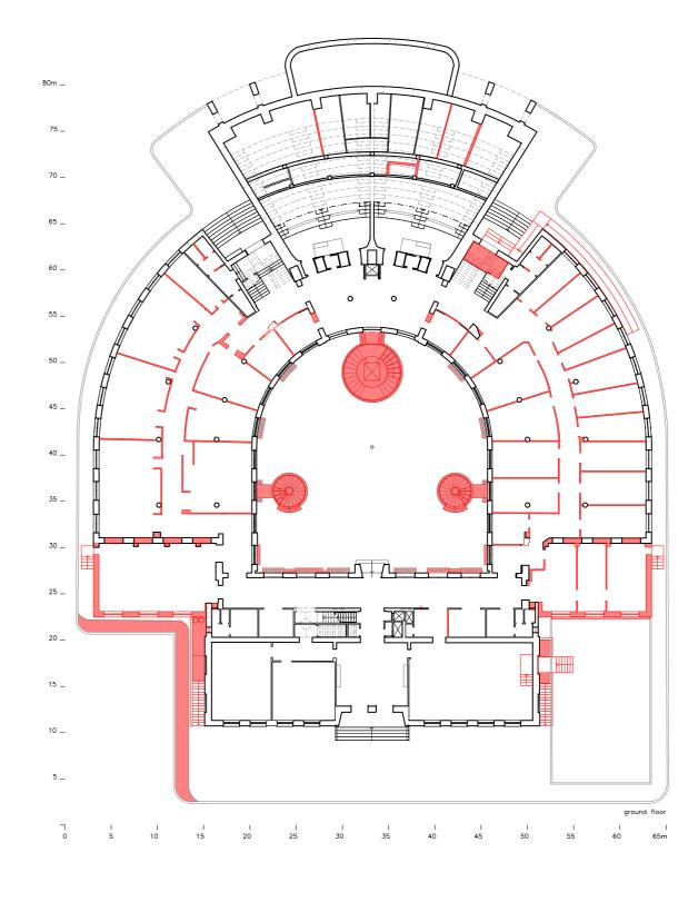
Figure 6 – Ground floor plan of the building; in red, additions from 1939 to the present day (© Cortesi 2021)
