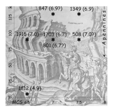
Figure 1 - Epicentral distance versus site intensity (IS > VI MCS); in brackets Mw values modified from CPT11. Note that the more severe effects in Rome derive from Apennines seismogenic earthquakes (BBL\_drw\_15)
