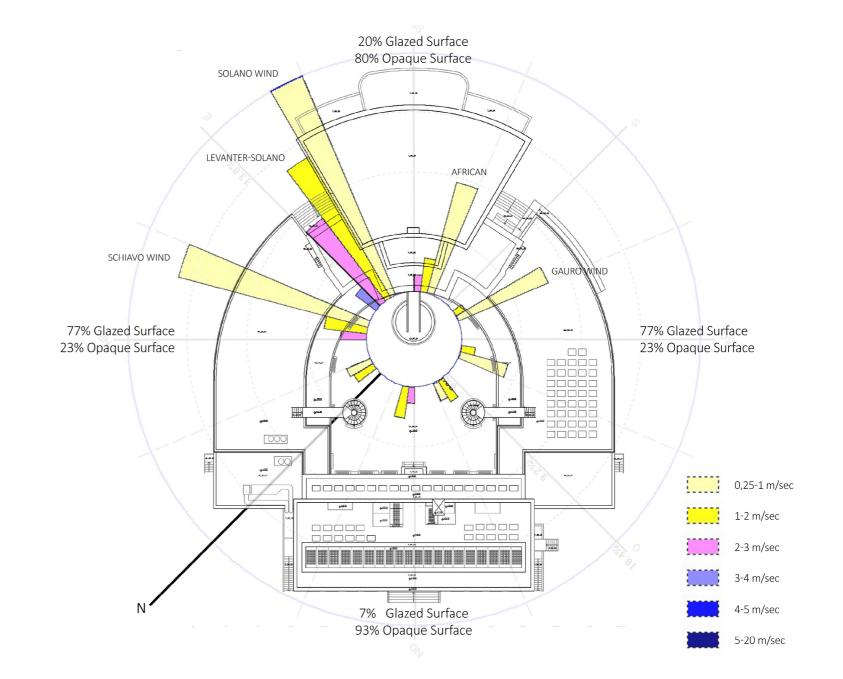
Figure 13 - Orientation diagram of the building, with percentage of opaque and glazed surfaces and prevailing compass wind rose (source of climatic data: http://www.arsial. it/portalearsial/agrometeo/E2\_5.asp year 2020)
