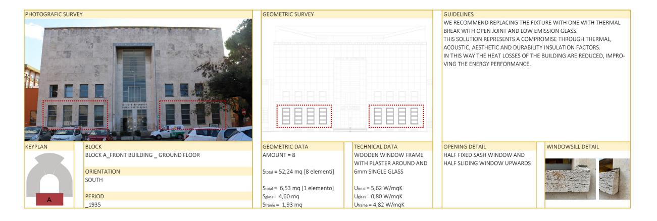
Figure 33 - Sample of analysis sheets of fixture types (© Romano 2020)
