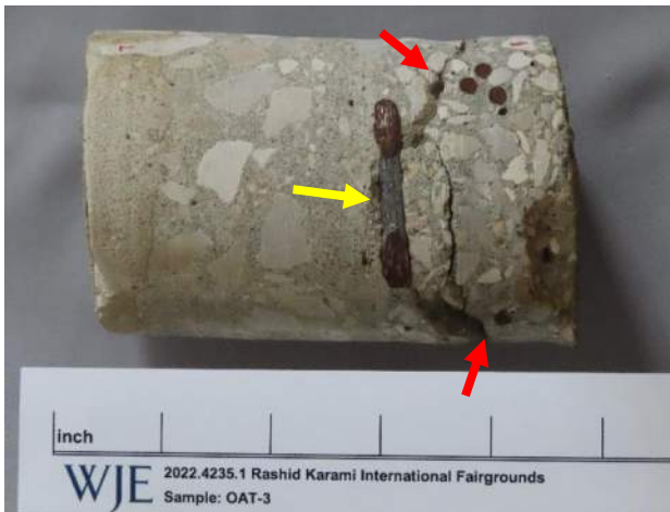
Figure 22. Core OAT-3 - Cracking (red arrows) adjacent reinforcement (yellow arrow) along interface of concretes.
