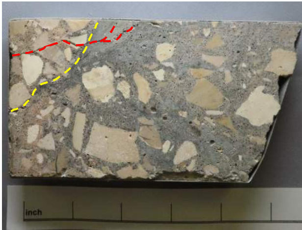
Figure 4. Core AR-2 - Lapped surface. The interface presumed to represent the construction joint is outlined by a yellow dashed line. A horizontal crack is marked with a red dashed line.
