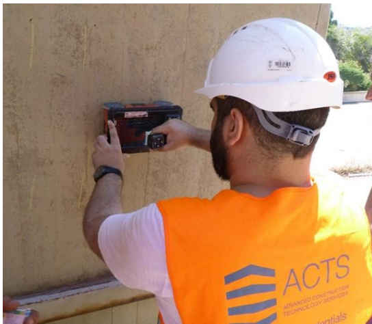
Figure 33. Nondestructive testing by Ground Penetration Radar (GPR) performed by ACTS on the Arch
