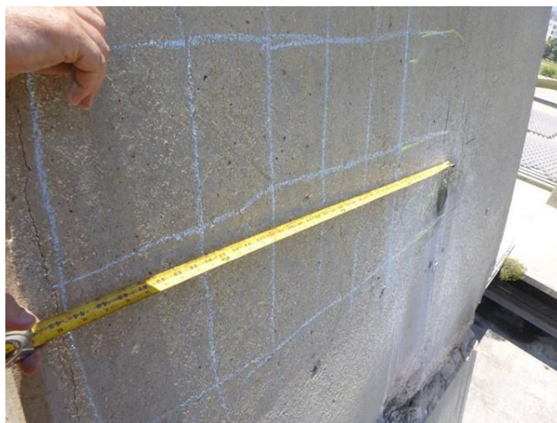
Figure 34. GPR scanning by ACTS on the Arch indicated the location of reinforcing steel in the concrete leg
