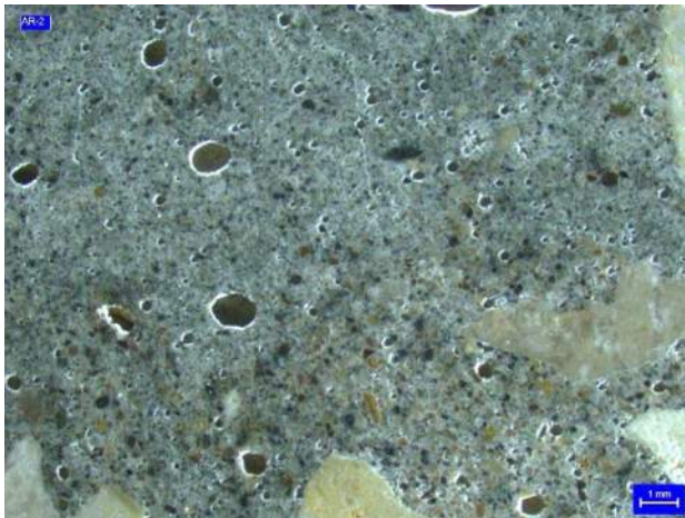
Figure 6. Core AR-2 - Light to dark gray mottling of the paste. Spherical and sub-spherical voids are visible.
