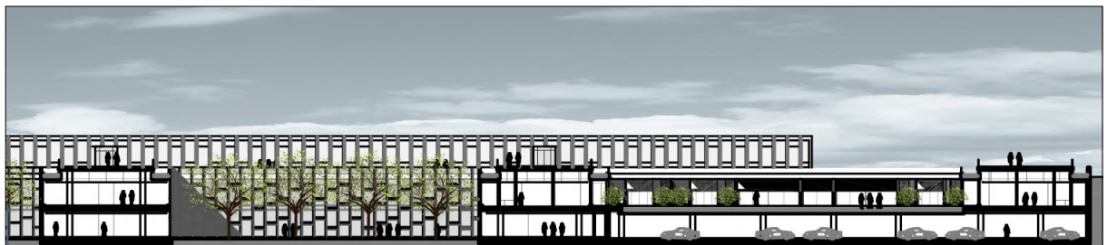
Section through the underground architecture by MDDM Architects. The interior was designed in a modular way rendering it highly flexible to the needs of the end-users.
