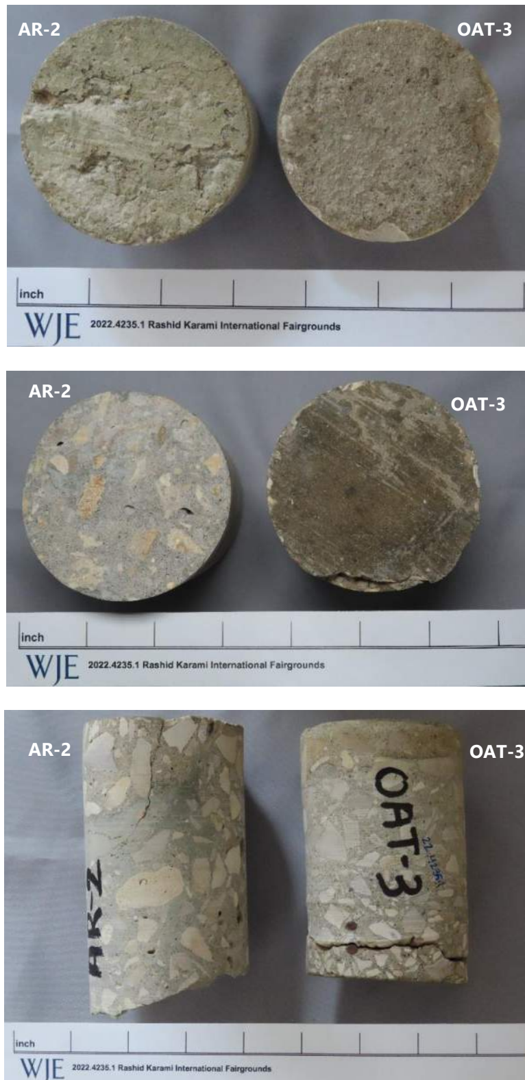
Figure 3. As-received appearance of the exterior/top (upper left), interior/bottom (upper right), and side of Core AR-2 (left in each image) and Core OAT-3 (right in each image).
