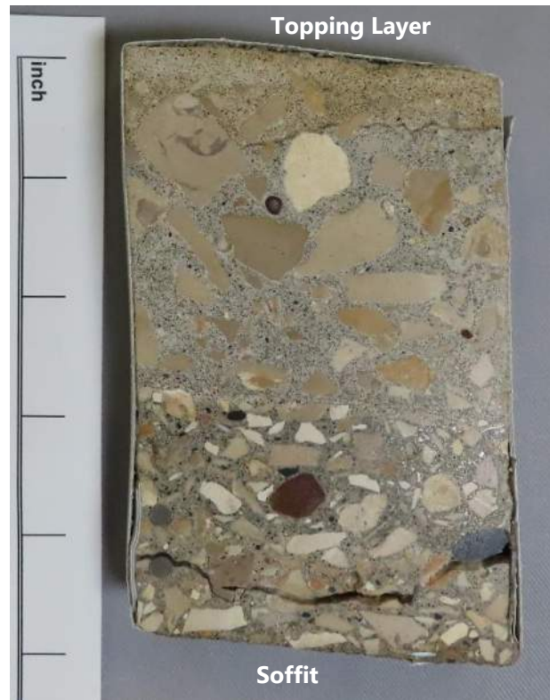
Figure 11. Core OAT-3 - Two concrete placements intersected by Core OAT-3.
