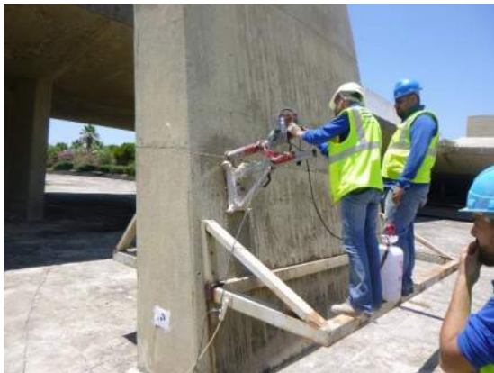
Figure 1. Core extraction of an Arch concrete sample used for laboratory testing.
