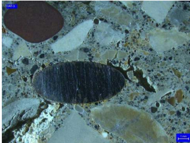
Figure 21. Core OAT-3 - Incomplete compaction of paste around reinforcement.
