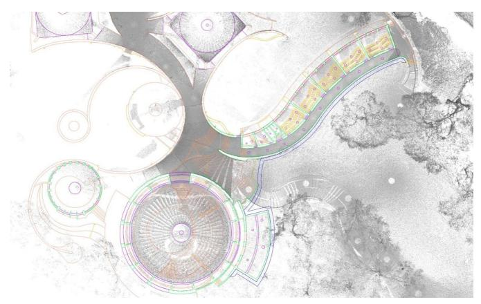
Figure 38 - Vector drawing of the School of Ballet overlapped to the georeferenced black and white cloud of points.
