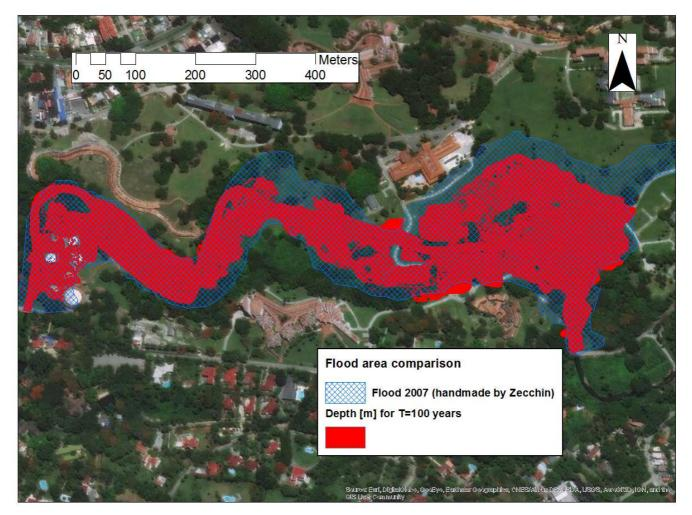
Figure 54 - Overlapping of the simulated maps with R = 100 years to the inundation sketch from the 2007 flood. In the red, flooded area in our simulation for R=100 years. In the gridded area, sketch of inundated area in 2007 flood.
