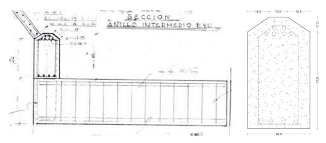
Figure 44 - The structural organization of the circular lower beam as indicated in the original design (left - ISA archive); drawing of the beam resulting from the on-site surveys (right).
