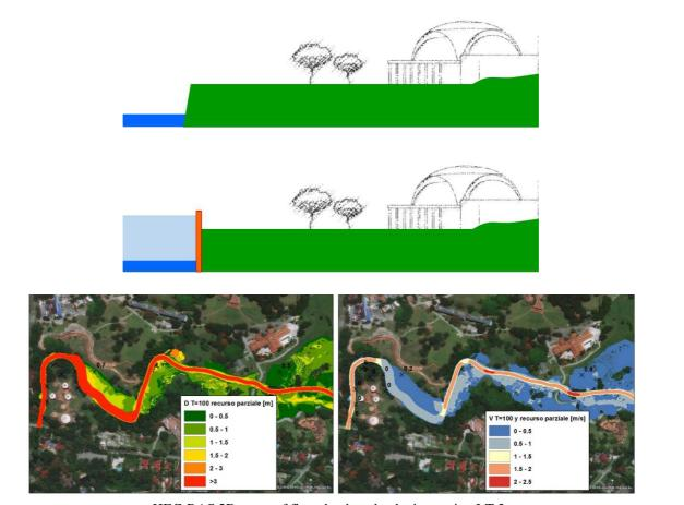
HEC-RAS 2D maps of flow depth and velocity, option LT.3. Possibly, channel widening as proposed by INRH is not necessary.
