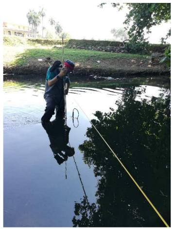
Figure 47 - Prof. Daniele Bocchiola of the Department of Civil and Environmental Engineering of Politecnico di Milano using a 2D flow tracker to estimate flow velocity, depth, and discharge in the Rio Quibù stream.
