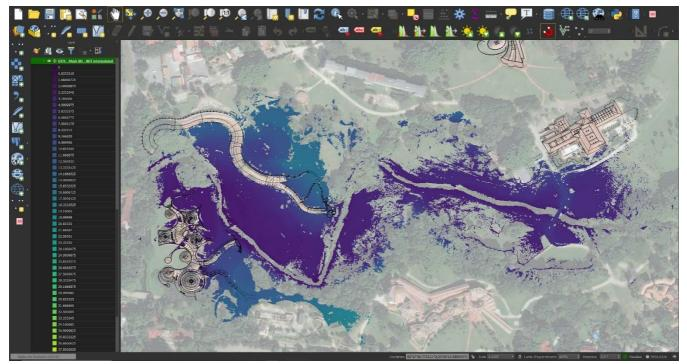
Figure 57 - Not interpolated Digital Terrain Model (DTM) on the Bing Virtual Earth map.
