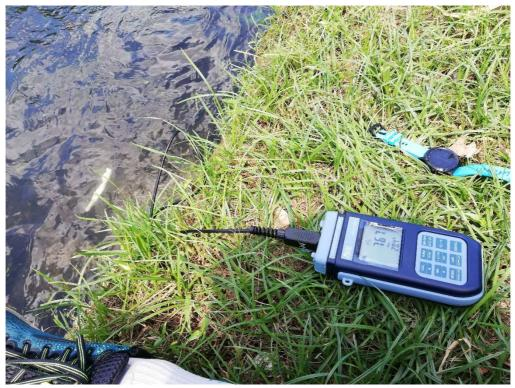
Figure 48 - Flow measurement in the Rio Quibù stream - salt tracer method.
