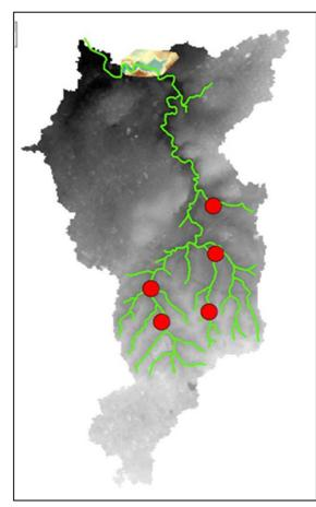
Figure 19 - Rio Quibù river catchment and synthetically derived hydrological network. Red dots are hydrometric stations potentially available. In color, the terminal area of the catchment with the School of Art, to be used as a domain for the hydraulic based flooding simulation. Resolution is 90 m, from ASTER.
