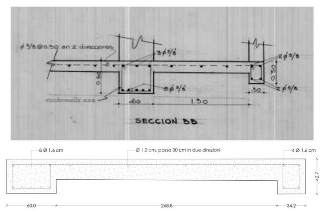
Figure 43 - The structural organization of the mezzanine. Above, the original design by Vittorio Garatti (ISA archive), below a drawing summarizing the results of the on-site surveys.
