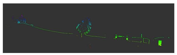
Figure 24 - East-West section of the cloud of points, the colors indicate the difference in altitude.
