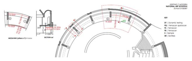
Figure 42 - Position of the tests performed on the mezzanine (from FB3254 to FS3264) nearby the pillar n.6.
