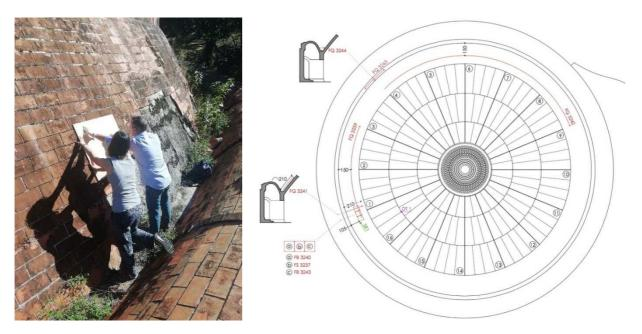
Figure 38 - The pacometer tests performed on the extrados of the Choreography Theater.
