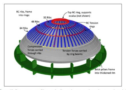
Figure 17: Dome structure in Rhino, with pillars and mezzanine depicted in green, dome shell in grey, ribs in blue, and tension rings in red. For ABAQUS analysis, pillars will not be included.
