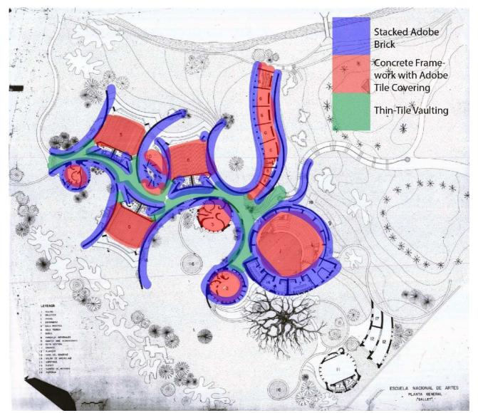
Figure 2 - Architectural plan of the School of Ballet with structural system types superimposed (image taken from Isabella Douglas bachelor thesis)
