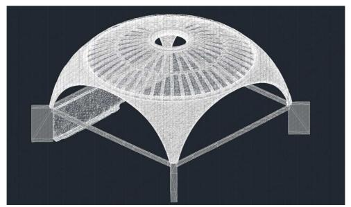
Figure 4 - Three-dimensional model of the Ballet School surveyed space (Zenith Ingegneria - Assorestauro associate).
