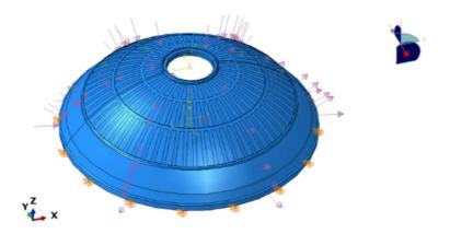
Figure 25: Wind loading on the Choreography Theater as visualized in ABAQUS, with purple arrows signifying the wind pressure into and out of the dome.
