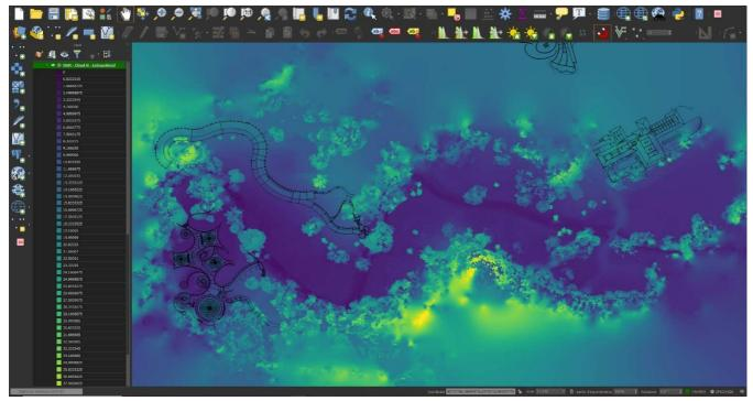
Figure 59 - Extrapolated Digital Surface Model (DSM).
