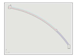
Figure 23: Locations of the reinforcement within the rib system body; dome shell is depicted in light blue, rib reinforcement is in red, crown reinforcement is in dark blue, and lower beam reinforcement is in dark green.
