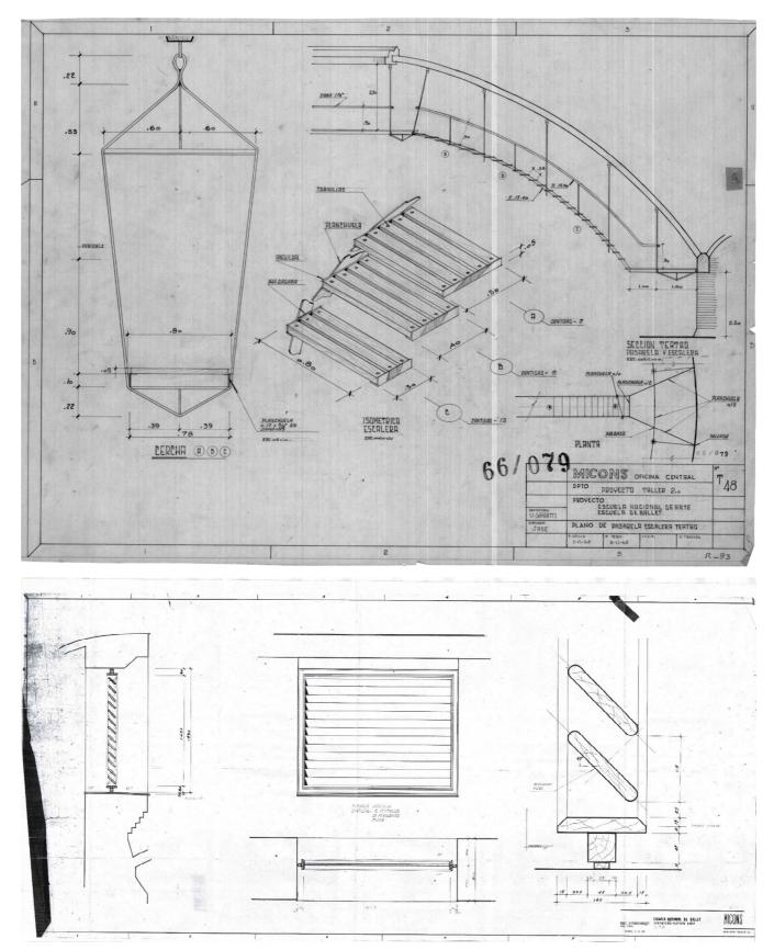
Figure 3 - Vittorio Garatti's original drawings for the School of Ballet. On top: the metallic catwalk of the Choreography Theater; on the bottom: the window frame for the Dance pavilions' changing rooms (ISA archive).
