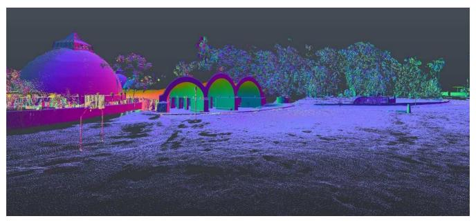
Figure 8 - Front perspective view of the "Union PA" point cloud with coloring depending on the plan variations.
