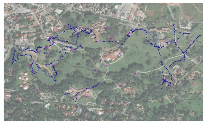
Figure 20 - "Bing VirtualEarth" aerial image, positioning of the 19 fixed GPS points (in pink) and the points acquired all over the area (in blue).
