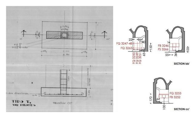
Figure 40 - The original drawings of the pillars (on the left - ISA archive) show the presence of a reinforced concrete core inside the masonry (20x40 cm, 1m high). On the right, the position of the tests carried out on the pillars.
