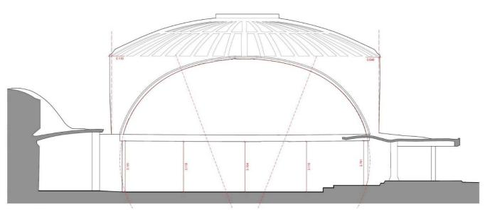
Figure 18 - Cross-section of the domed space of the Ballet School with dimensions and outlines.
