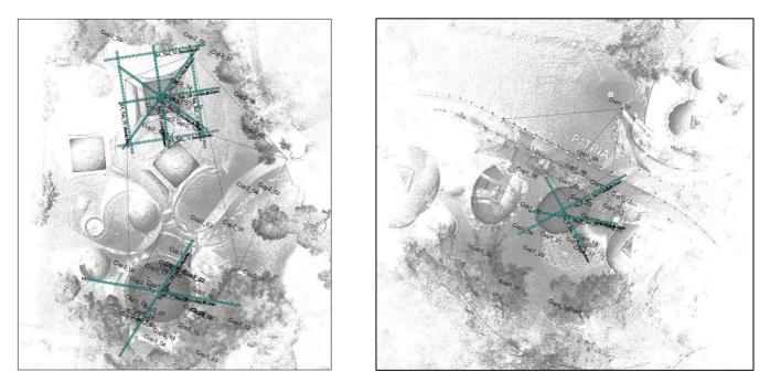
Figure 12 - Point cloud of the School of Ballet, zenith projection; Figure 13 - Point cloud of the School of Plastic Arts classroom, zenith projection.
