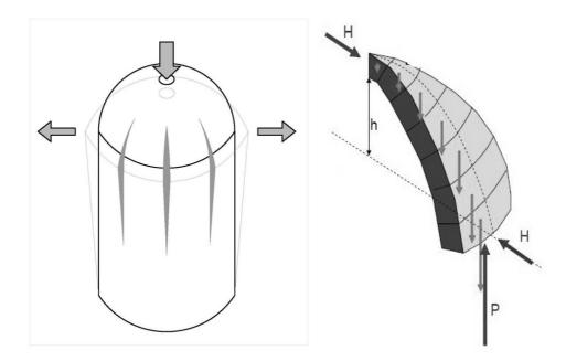
Figure 65 - On the left, the damage mechanism typical of (masonry) domes; on the right the macro-elements calculation in the simplified analysis as "arches" with Mery's graphic method and in the equilibrium approach.
