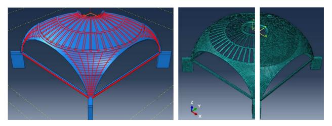
Figure 81 - Reinforcing bars and shells embedded within solid parts (left) and meshed models (center and right).
