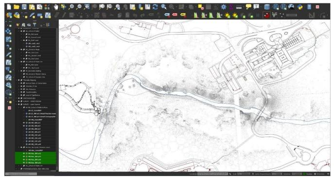
Figure 62 - Grayscale cloud of points of the central area of the ISA.
