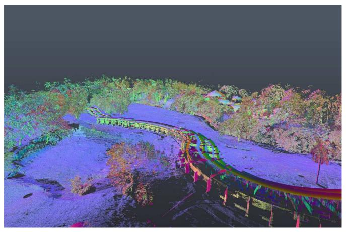
Figure 4 - Perspective view of the point cloud "Union BA\_MU" with coloring determined by plan variations.
