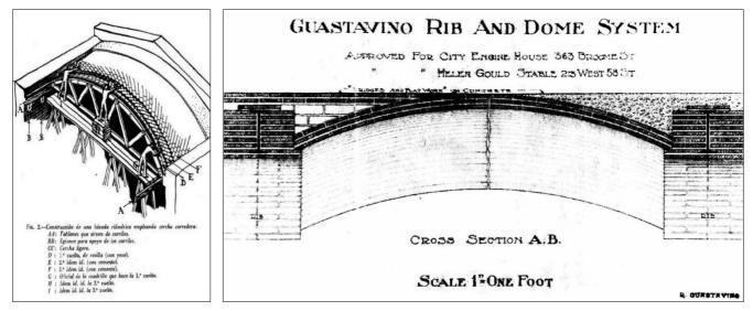
Figure 92 - On the left: Illustration of the construction process of catalan vaults (from L. Moya Blanco, Bovedas Tabicadas, Ministerio de la Gobernacion - Direccion generale de Arquitectura, 1947, p. 20). On the right: Guastavino's "Rib and Dome system" (from J. Parks, A. Neumann, The old world builds the new, Biblioteca Avery, 1996).
