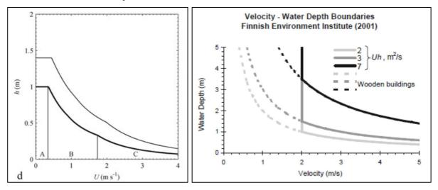
Figure 63 - Left: Stability thresholds for adults (thin line) and children (thick line), found out by Milanesi et al. (2015); right: Empirical criterion for damages to buildings of the Finnish Environment Institute—FEI (Maijala 2001): masonry buildings are the continuous lines.
