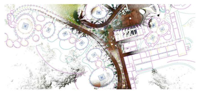
Figure 39 - Vector drawing of the School of Plastic Arts overlapped to the georeferenced colored cloud of points.
