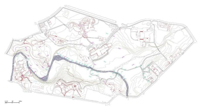
Figure 9 - General plan of the ISA with the location of the scan points (in green, the scans registered in grayscale, color scans are in purple).
