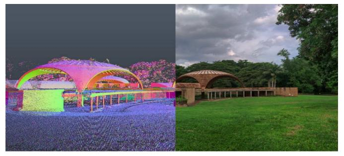
Figure 5 - Perspective view of the School of Ballet. On the left: a cloud of points with coloring determined by the plan variations. On the right: spherical color image.
