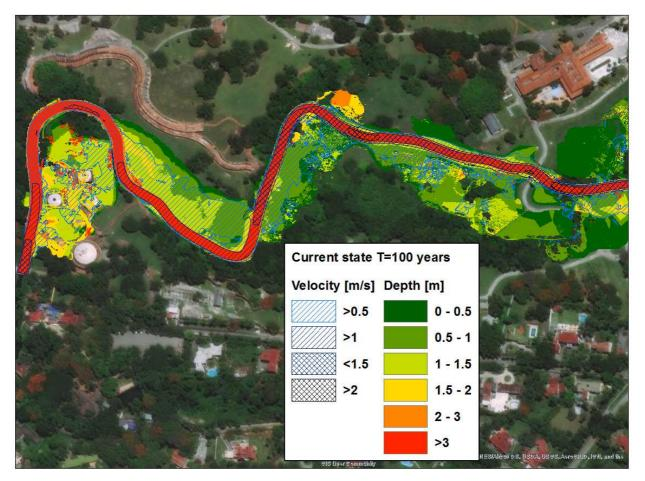
Figure 56 - Integrated scenario based on velocity and water depth (Return period 100 years) from HEC-RAS 2D.
