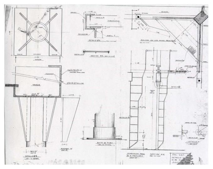
Figure 56 – Original drawing illustrating the details of the metallic pillars and balconies (ISA archive)
