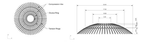
Figure 20: Rib reinforcement shell with dimensions, modeled as a surface with no thickness in Rhino
