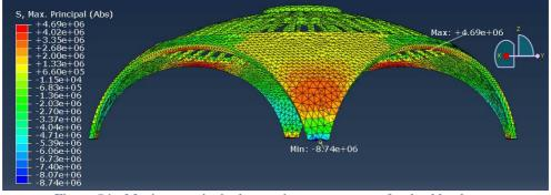
Figure 84 - Maximum principal stress in superstructure for dead load case.
