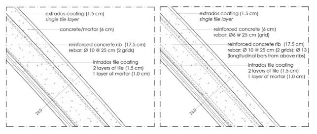
Figure 39 - Stratigraphy of the crown located at the base of the Choreography Theater. On the left: main rebar arrangement; on the right: rebar arrangement at ribs continuation.
