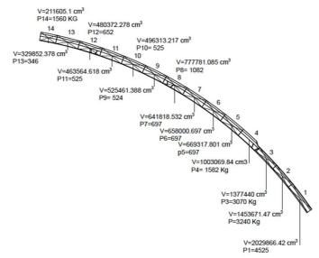
Figure 66 - An "arch-slice" of the dome, which simulates the behavior of the continuous ribs. The arch is divided in 14 elements, whose volume (V) and weight (P) are reported in the figure, for the successive Mery's graphic analysis.
