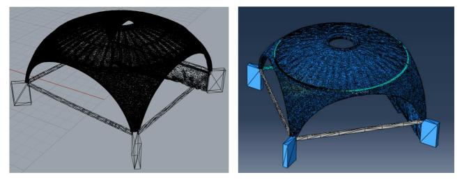
Figure 80 - Laser scan geometric (left) and meshed (right) models.
