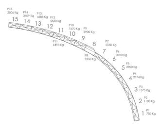
Figure 77 - The diagonal "arch-slice" representing ¼ of the dome. The arch is divided in 15 elements, whose weight (P), used for the successive Mery's analysis, are plotted in the figure.
