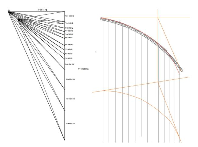
Figure 67 - On the left, the two polygons of forces with the fictitious pole (O') and the real one (O) from which the inclination of the line of thrust inside the dome can be obtained (right).
