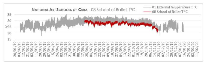
Table 16 - Temperature data T° Sensor 08 in the School of Ballet, compared to the outside temperature.
