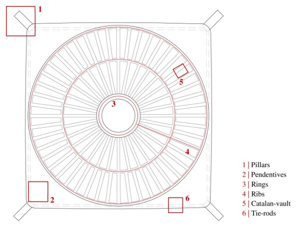
Figure 52 - Outline of the main constructive elements composing the Pavilion Dome of Practical Room (BA.3.59).
