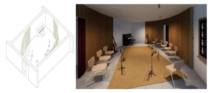
Figure 73 - Panel: Modular acoustic panel system. Basement classroom application.
