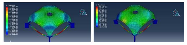
Figure 82 - Deflection magnitude in meters under dead load (left) and under wind load (right).
