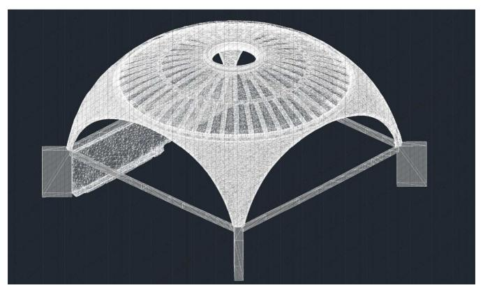
Figure 16 - Three-dimensional model of the Ballet School surveyed space.
