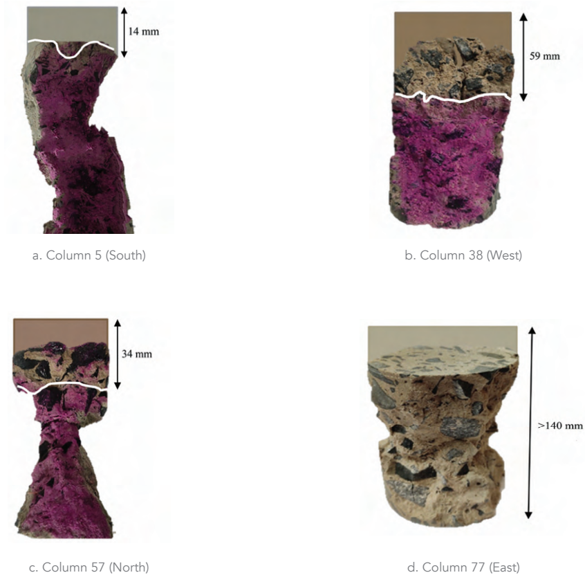
Fig. 96: Carbonation depth in concrete (Note: The extended grey region is the ground concrete part from the concrete core. The grinding was done to enable the Compressive Strength testing.)
