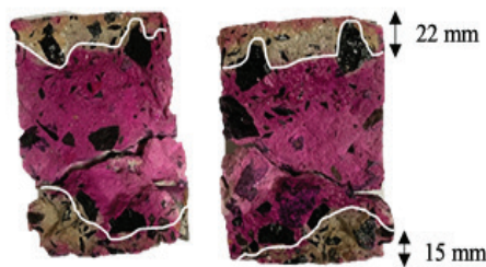
Fig. 105: Carbonation of concrete in the canopy
