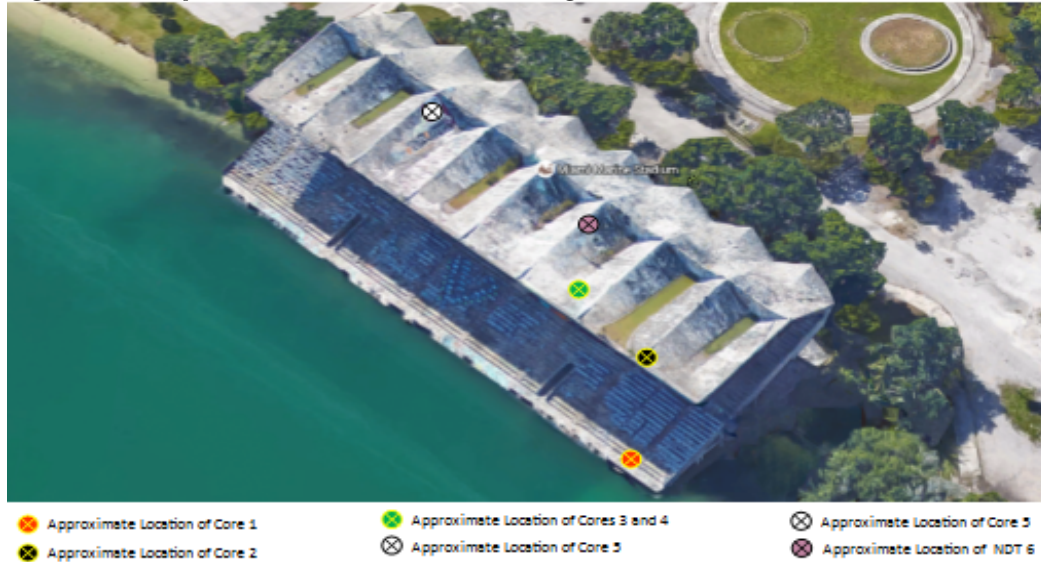
Figure 1: Sample extraction and NDT testing locations
