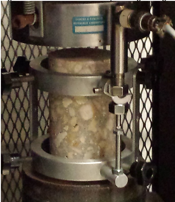
Figure 2: Modulus of Elasticity testing configuration
