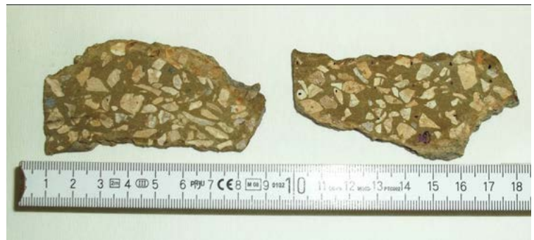
Figure 33: General view of the yellow-colored concrete mosaic slab used as floor finishing at the courtyard (on the left) and the cross section of concrete mosaic sample (C8.E.E4.) (on the right)
