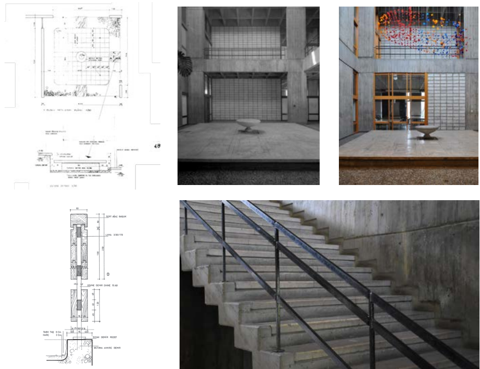
Figure 103: The actual design and current form of the Göbektaş area and the balustrades.
