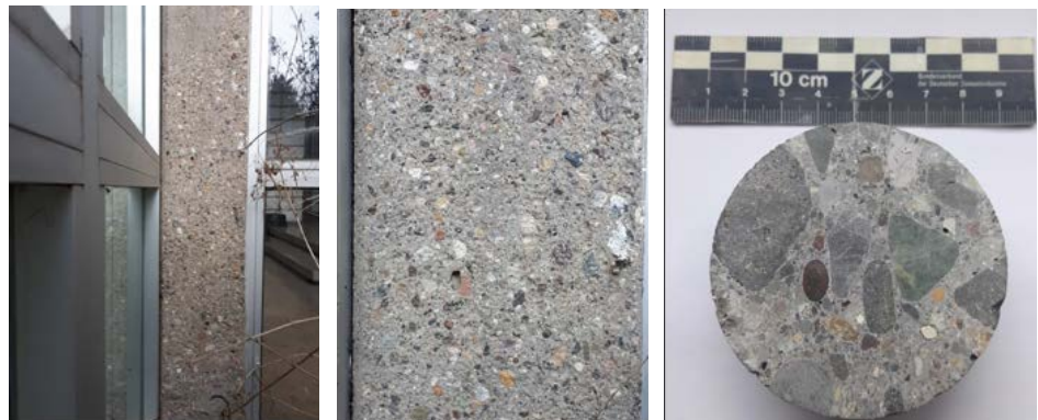
Figure 19: General view of the exposed concrete wall (on the left) and the cross section of the exposed concrete core sample (C3.X). (on the right).
