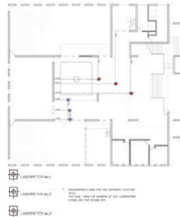
Figure 37: Location of laser meters.
