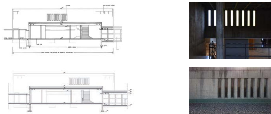
Figure 104: The changing position of the windows on the north façade of the F Block, the interior and exterior view of the current condition
