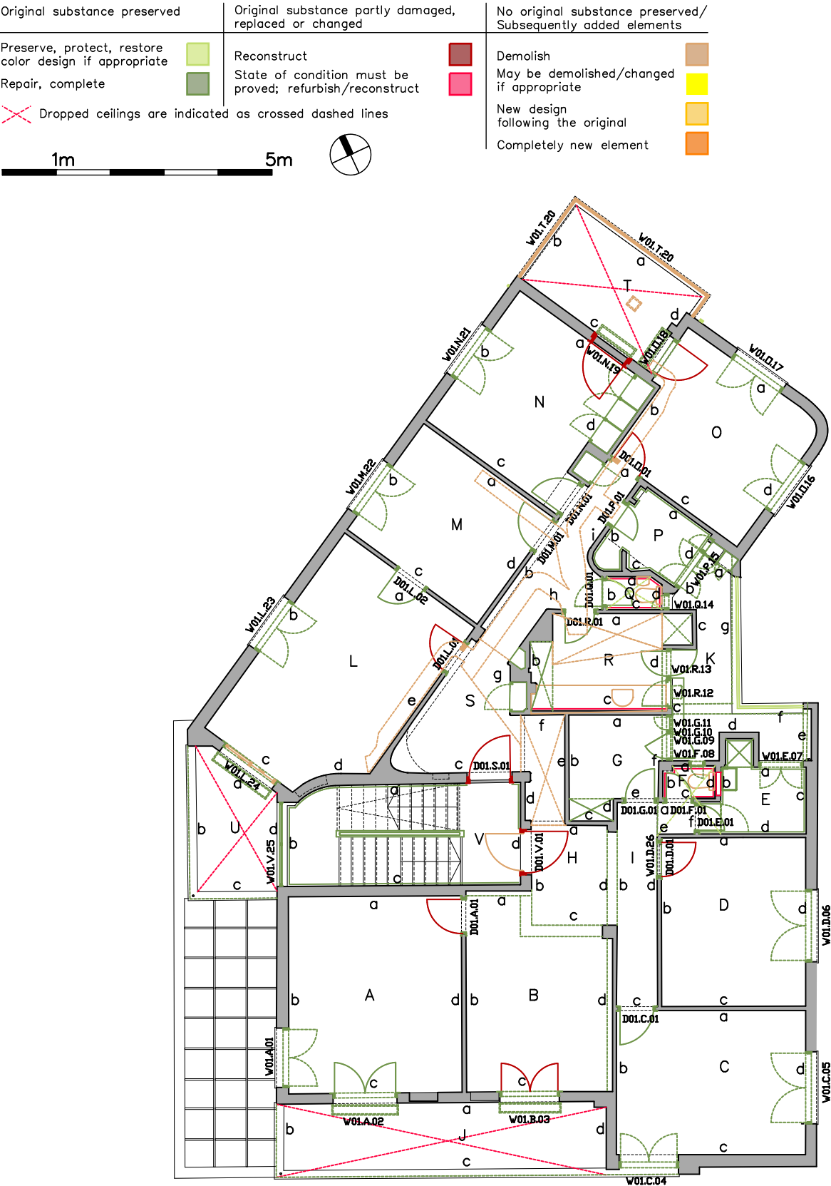
Fig. 47 Preservation measures, fixtures, built-in furniture, 2nd floor
