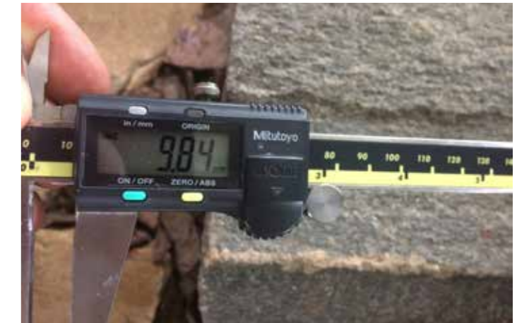
Image 3: Reading the thickness of the tube on the calipers
