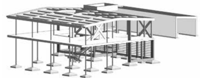
Figure 4: 3D view of structural modeling
