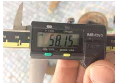
Image 9: Measurement of slab thickness
