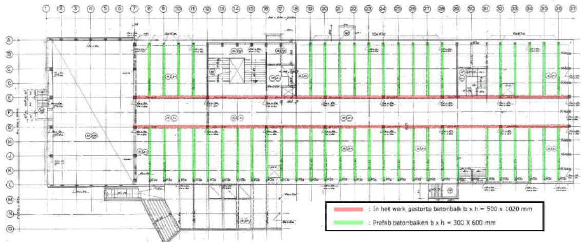
12. Principle beam system, image ABT
