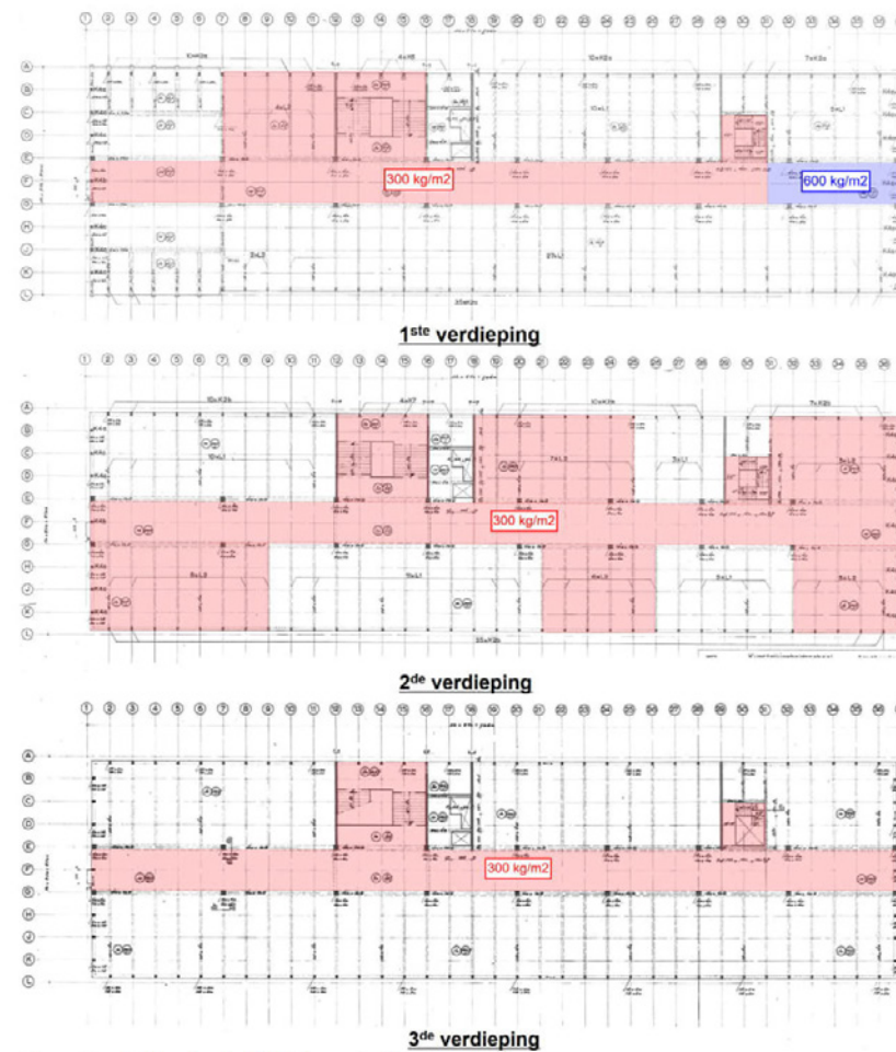
14. Different floor loads 2nd to 4th floor, image ABT
