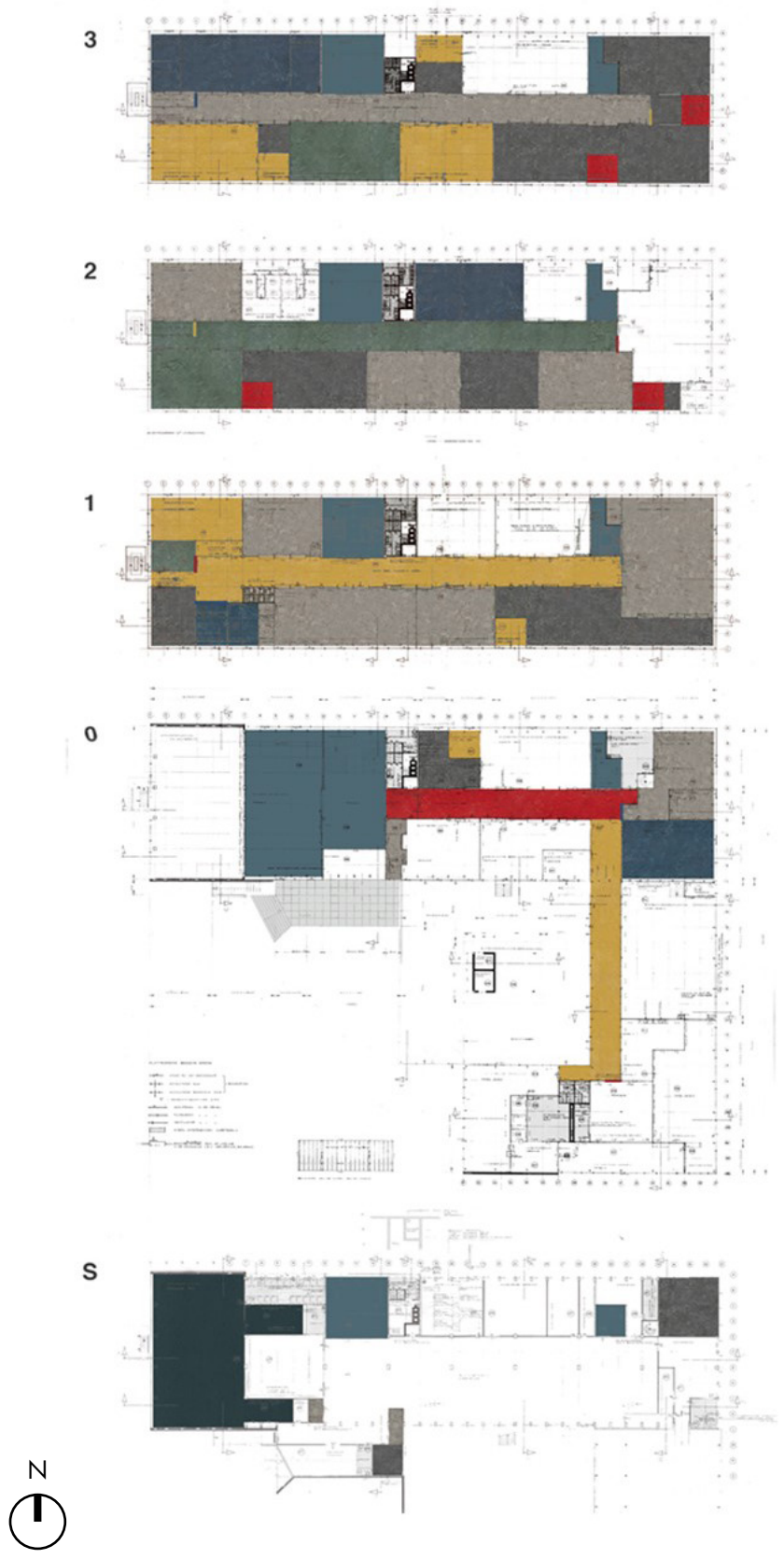
35. Floor plans with marmoleum, cork linoleum and plasnalo floor finishes
