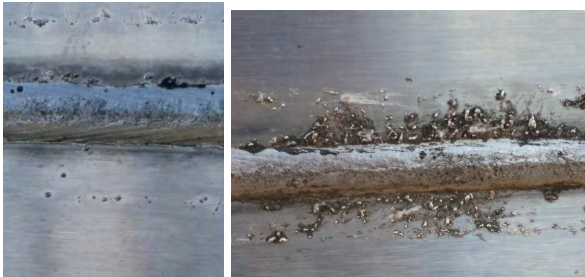
Figure C11 and C12: Weld spatter differences in areas with minimal versus significant surface deposits. (Photos taken by authors in 2014)
