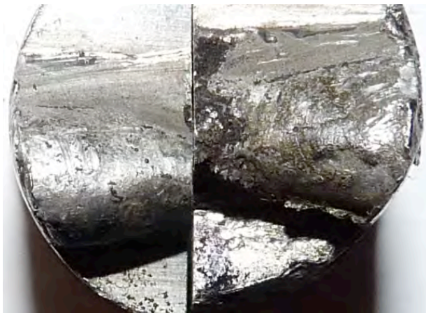
Figure A35: W5 after sectioning through weld slag contamination that was visible on the weld surface. (Photo taken by authors in 2014)
