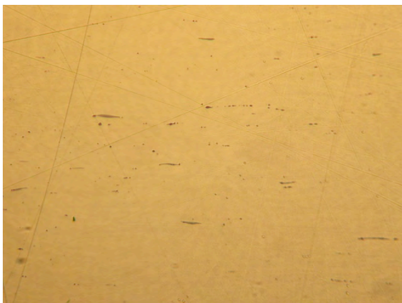
Figure A7: Micrograph of manganese sulfide stringers in the plate, W1, as-polished condition. (256x) (Photo taken by authors in 2014)
