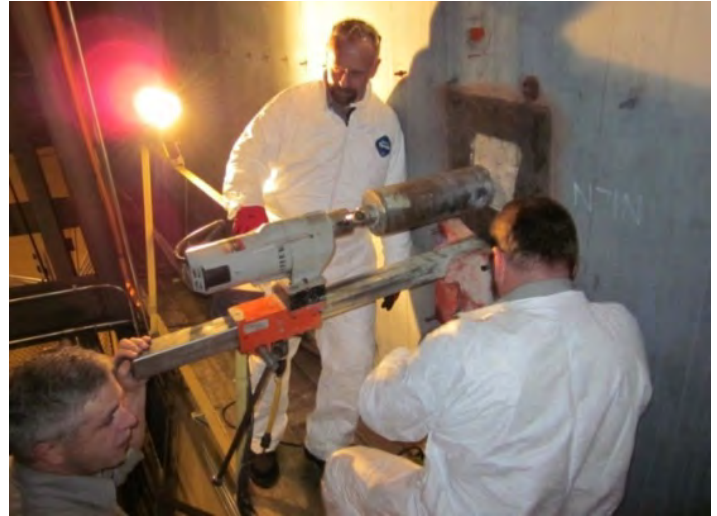
Figure 2-29—Coring extraction of 5 inch diameter concrete sample using a coring rig attached to the wall at North Station 71. Source: S. Kelley
