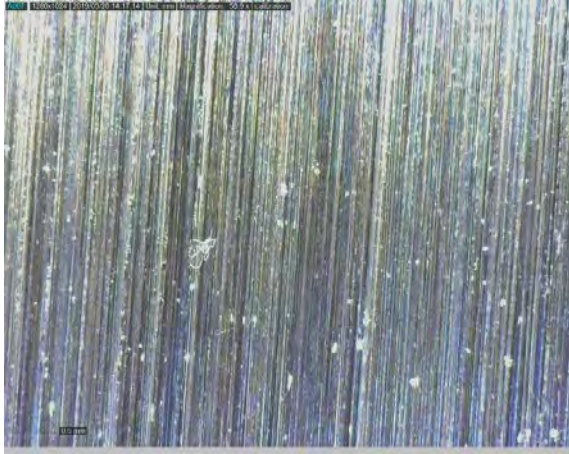
H.2 Sample Astropak #7 hand buffed images: (L) Deicing salts staining was completely removed with some minor surface pitting observed 58.9x, (R) This area was particularly aggressively scratched. Some very small embedded iron particles and resultant staining were still present on the surface but only visible under microscopic examination 59x.
