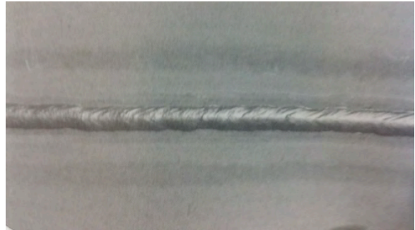
Figure B1: Ideal stainless steel weld appearance (Photo taken by authors, archive)
