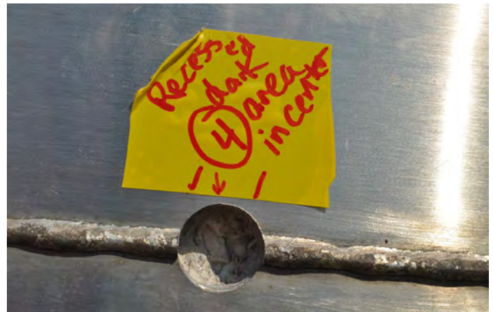
Figure 2-34—Removal of a field weld sample from the exterior skin of the arch. Source: S. Kelley
