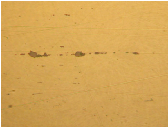
Figure A6: Micrograph of a plate inclusion, W1, as-polished condition. (517x) (Photo taken by authors in 2014)
