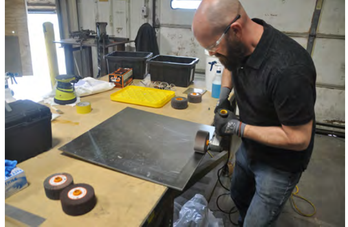
Figure 5-64: Using a cylindrical sander to refinish one of the panels with incised graffiti. Source: S. Kelley
