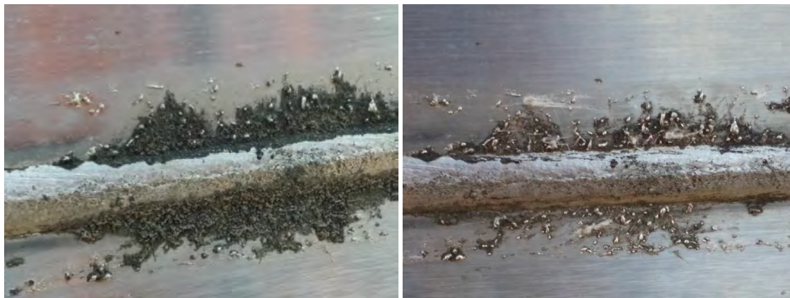
Figures C1 and C2: Dark deposit accumulation around and extrados weld, before collection of sample 2B (C1, left) and after sample collection and additional cleaning with an alcohol dampened cloth (C2, right). (Photo taken by authors in 2014)
