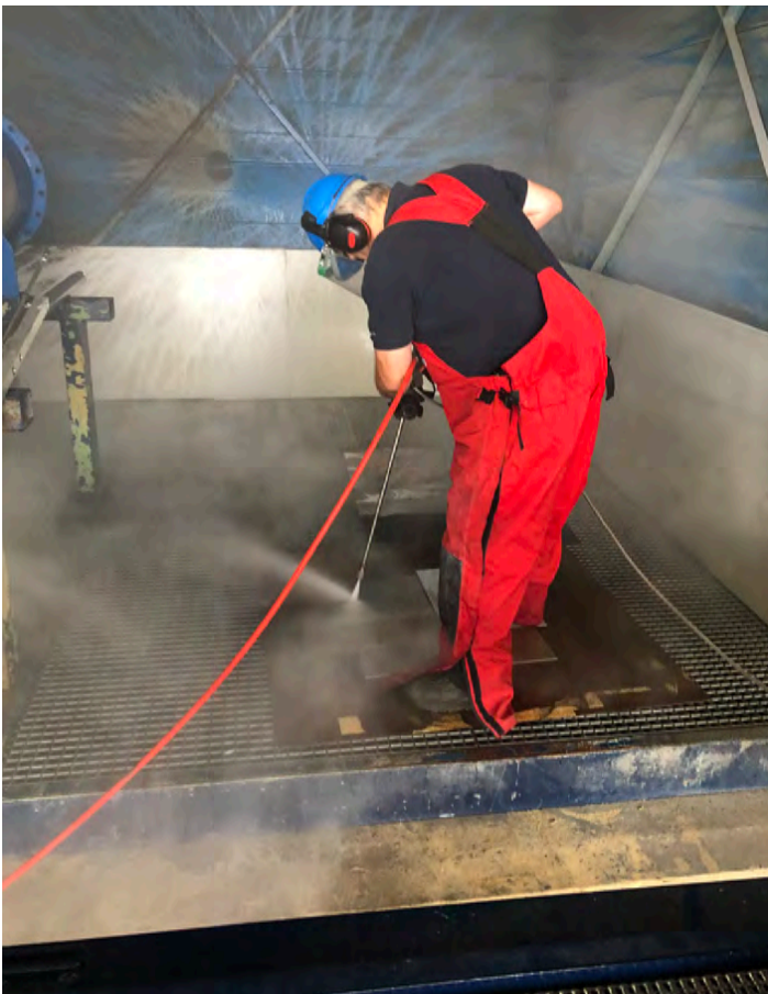
Figure 5-29—Test 6B-1 ultrahigh pressure (1500) water cleaning by Kärcher and their facility in Germany. Source: Kärcher
