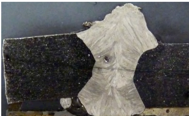
Figure A32: Macrograph W5 etched condition with a visible void. The minor plate misalignment
