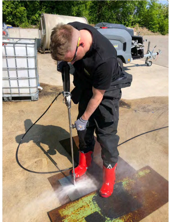
Figure 5-28—Test 6A ultrahigh pressure (1000 bar) water cleaning by Kärcher at their facility in Germany. Source: Kärcher
