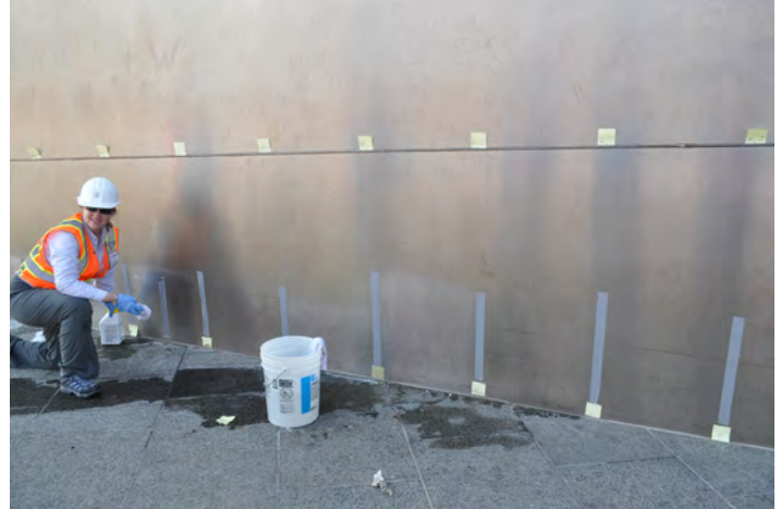
Figure 5-47—Testing being performed using mild chemical/abrasive methods on the east face of the north leg of the monument in 2014. The technician is Catherine Houska. Source: S. Kelley
