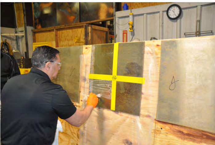
Figure 5-37—Application of the rouging compound with a paintbrush. Source: S. Kelley
