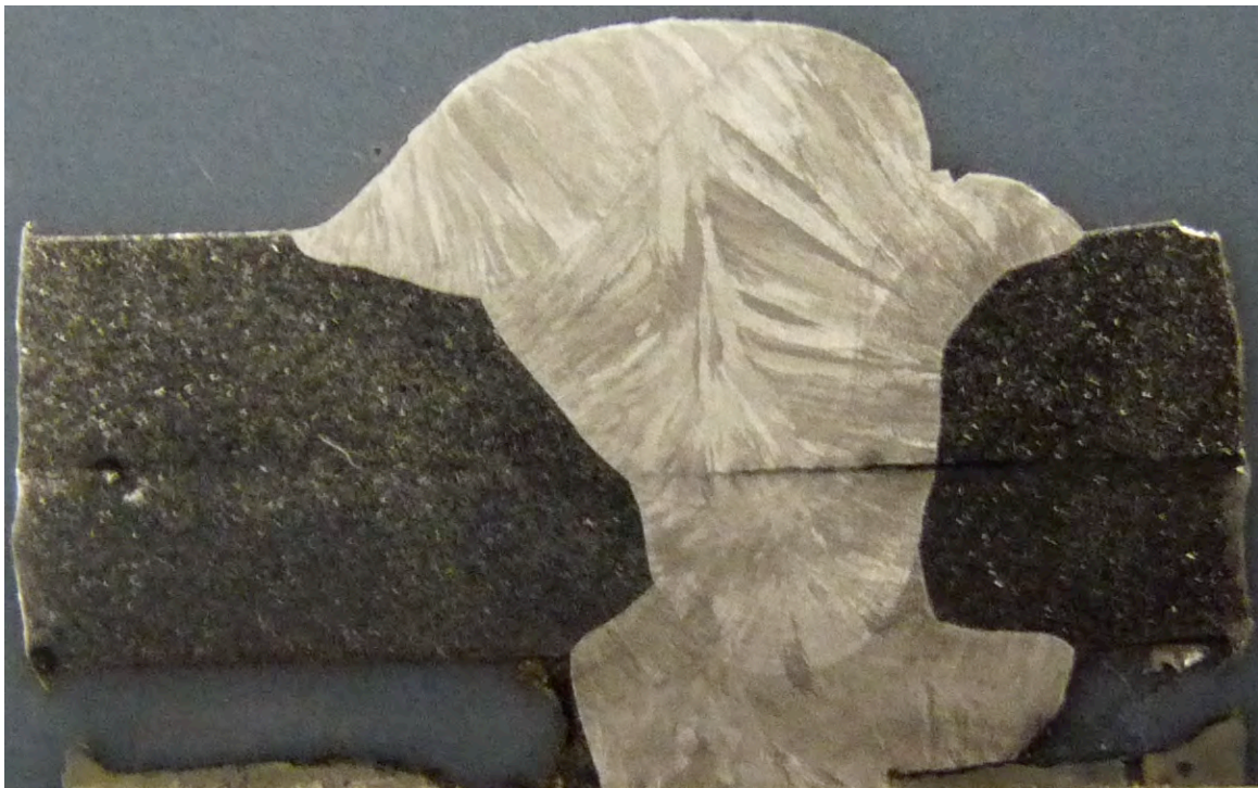
Figure A19: Macrograph of W3, etched condition. (Photo taken by authors in 2014)
