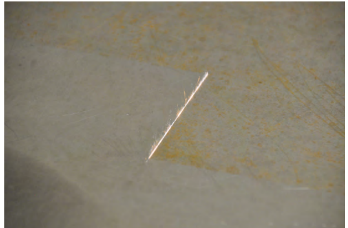
Figure 5-45—Close up view of the laser cleaning showing the immediate results. Source: S. Kelley
