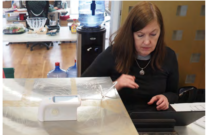
Figure 5-53—Using a MeterTo 3nh Tri Gloss meter to measure spectral gloss. Source: D. Worth
