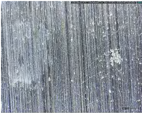
H.3 Sample Astropak #9 hand buffed bottom images: (L) Deicing salts staining was completely removed. This sample had numerous areas with the unidentified surface deposit, which is also shown in this image. 58.8x, (R) No embedded iron particles were observed but some residual staining was still present on the surface. The unidentified deposit appeared to be holding these remaining particles onto the surface, so the cleaning method was considered effective in meeting the goals of the project. The effect of the deposit was only clearly visible under microscopic examination. 59.3x.
