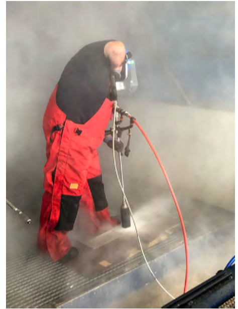
Figure 5-32—ultrahigh pressure (1500) water cleaning using a round nozzle by Kärcher and their facility in Germany. Source: Kärcher
