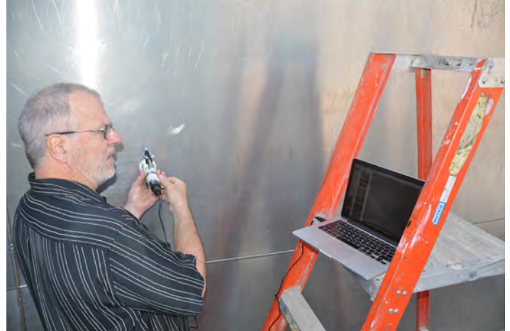
Figure 5-16—Examination of the stainless steel skin utilizing digital microscopy. Source: S. Kelley
