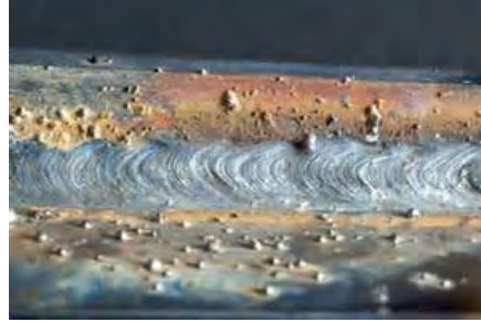
Figure B3: Weld spatter. (Photo Avesta Welding Manual)
