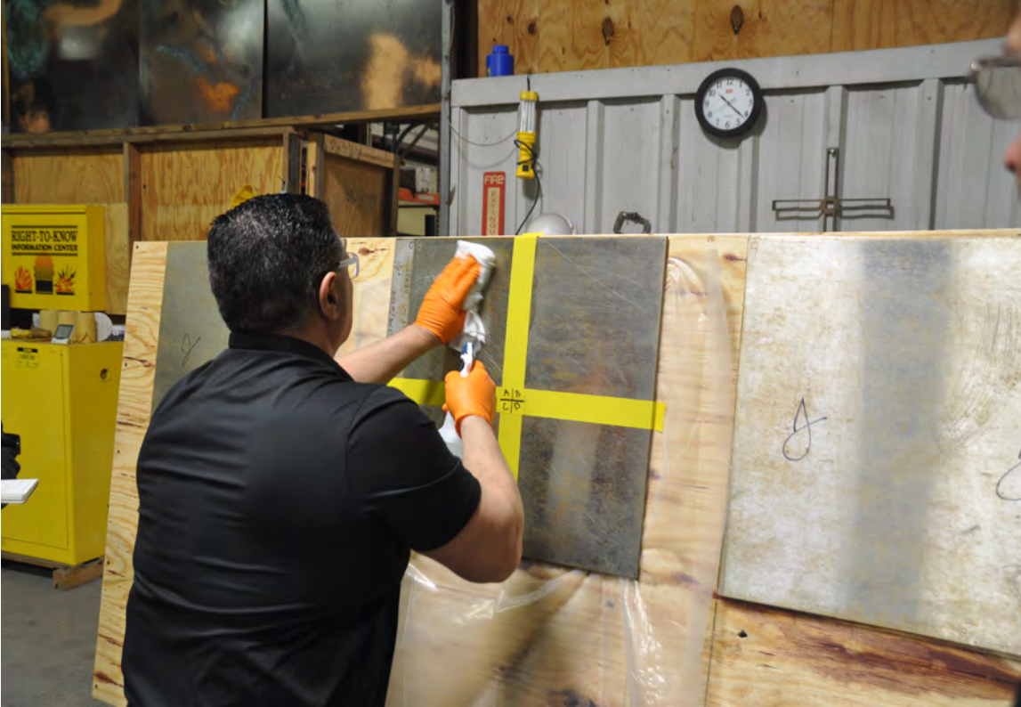
Figure 5-36—Wiping of the surface of the panel with isopropyl alcohol and a cotton cloth to remove film and other debris.
