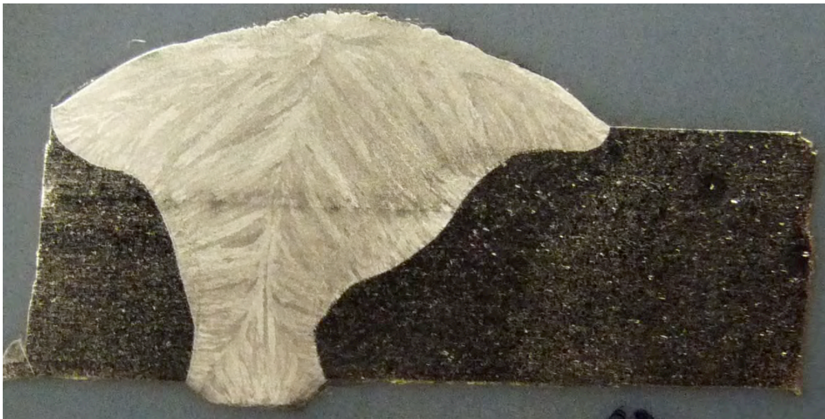
Figure A3: Macrograph cross of section W1 in the etched condition (Photo taken by authors in 2014)
