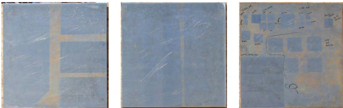
Figure 5-45—Close up view of the laser cleaning showing the immediate results. Source: S. Kelley
