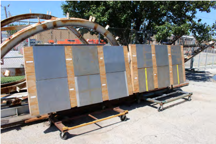
Figure 5-50—The test panels showing water, dry ice, chemical and laser cleaning techniques located outside during a sunny day for visual (aesthetic) assessment. Source: J. Cawby
