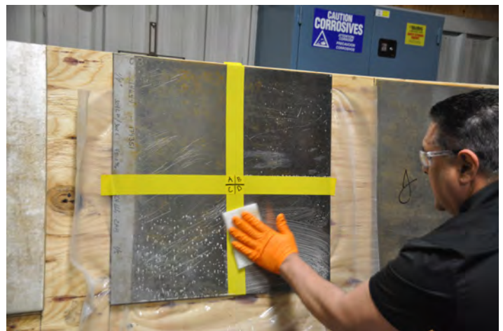
Figure 5-38—Vigorous scrubbing of the surface by hand using a Scotch Brite pad. Source: S. Kelley
