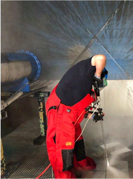
Figure 5-30—Test 6B-2 ultrahigh pressure (2200) water cleaning by Kärcher and their facility in Germany. Source: Kärcher
