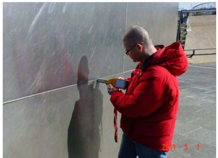
Figure 2-28—The surface of the steel was evaluated using a handheld XRF in March 2011. Source: P. Krauss
