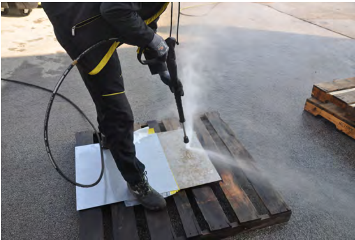
Figure 5-26—Test 4A ultrahigh pressure (500 bar) water cleaning by Kärcher. Source: S. Kelley
