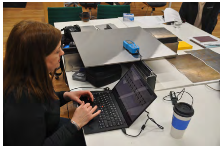
Figure 5-54—Using a VTSYIQI SurfTest KR200 Portable Profilometer to measure surface roughness. Source: S. Kelley
