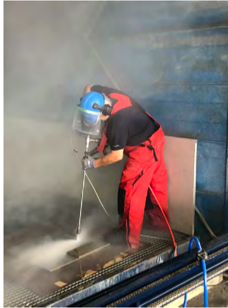
Figure 5-31—Test 6B-3 ultrahigh pressure (3000) water cleaning by Kärcher and their facility in Germany. Source: Kärcher
