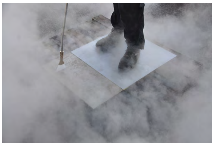
Figure 5-25—Test 3B steam cleaning by Kärcher. Source: S. Kelley
