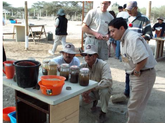
Figure 3.2.3 PAT students performing in-situ sedimentation test PAT course, 1999 © J. Paul Getty Trust
