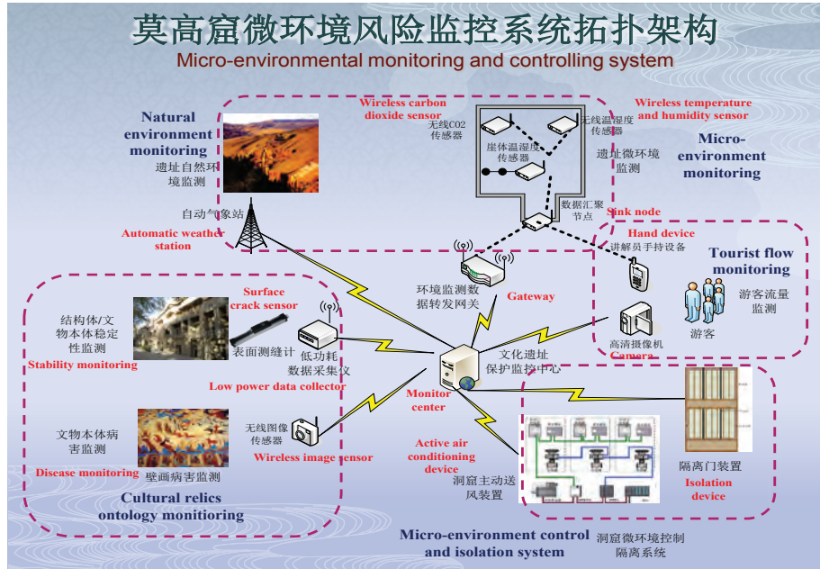
Fig. 7. The framework of the micro-environmental monitoring and controlling system at the Mogao Grottoes
