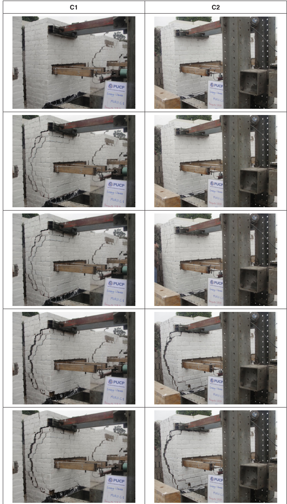
FIGURE 6.20. Crack propagation during testing of type C specimens.
