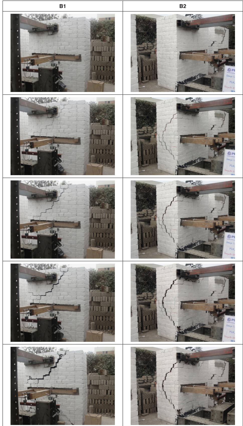
FIGURE 6.19. Crack propagation during testing of type B specimens.
