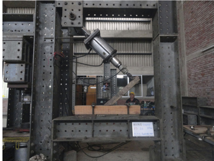
FIGURE 5.5. Test setup for the nailed connection between post and diagonal bracing.
