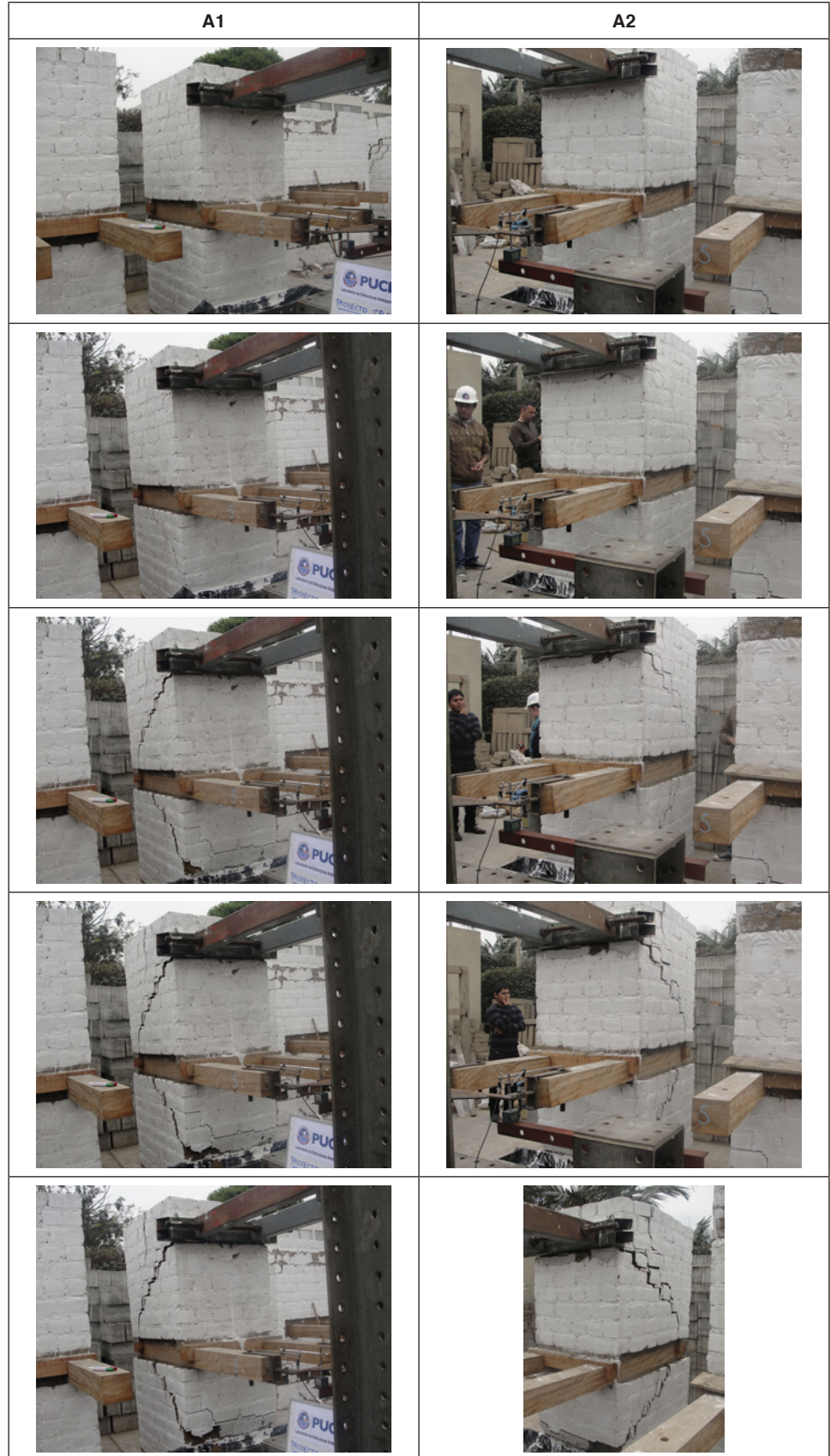
FIGURE 6.18. Crack propagation during testing of type A specimens.
