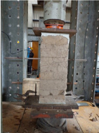
FIGURE 2.8. Compression test on adobe pile. Vertical cracks are visible in the units and the mortar.
