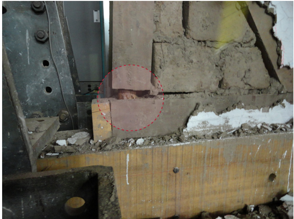
FIGURE 4.14. Image showing the tenon lifting from the mortise (red circle) at maximum horizontal displacement of specimen MA.
