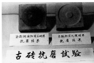
Figure 2 Sample tiles from Meridian Gate after abrasion-resistance testing with raw tung oil; treated tile on left and untreated tile on right.
