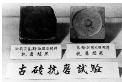
Figure 1 Sample tiles from Meridian Gate, Beijing Palace Museum, after abrasion-resistance testing; tile consolidated with polyurethane on the left and untreated tile on the right.
