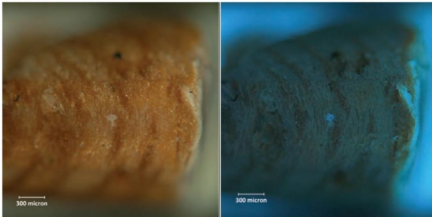
**Figure 25. Sample 43 from NO6H, cross sectional view under visible (left) and UV illumination.**
