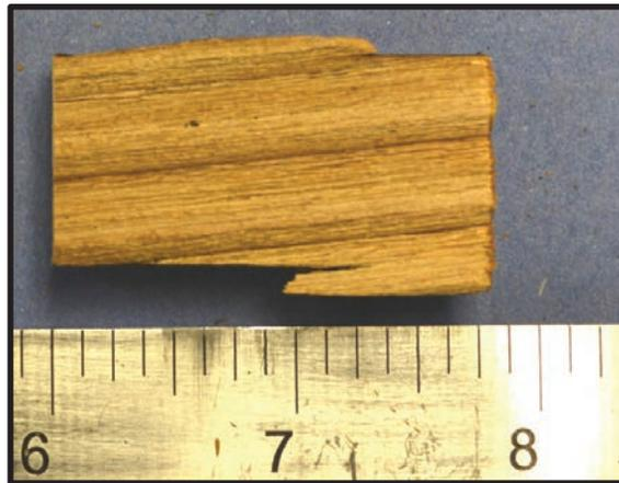
**Figure 4.23.** Small portion of specimen C showing extensive erosion of the earlywood on the exposed face.
