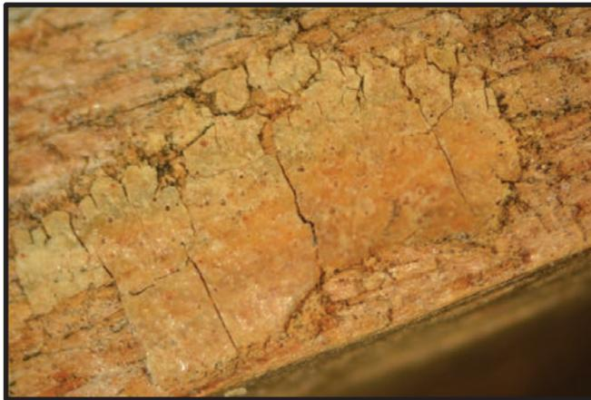
**Figure 4.5.** Specimen G showing remnants of an adhesive on the side face.
