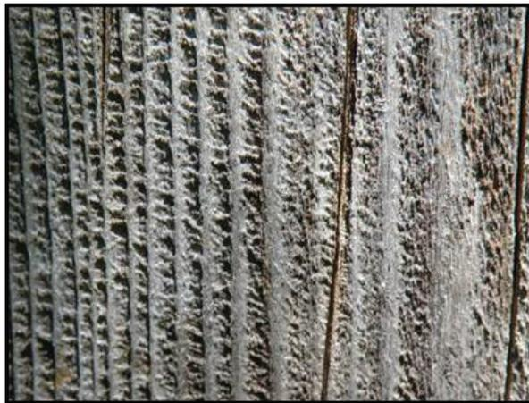
**Figure 2.1.** Example of an uncoated wood substrate with natural erosion of the lower-density earlywood due to weathering.
