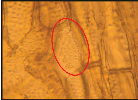
**Figure 4.17.** Alternate intervessel pitting, specimen F, 400x magnification.
