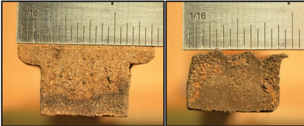
**Figure 3.9.** (Left) Specimen C, top end grain prior to sanding; (right) Specimen C, bottom end grain prior to sanding.
