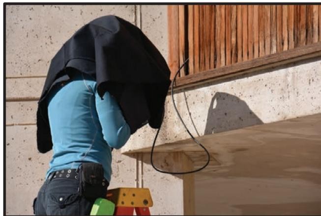
**Figure 3.4.** Use of the videoscope to determine wall cavity conditions.
