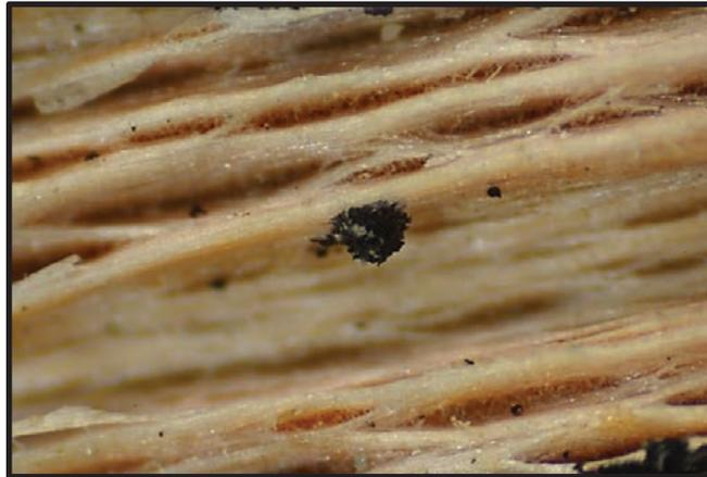
**Figure 4.3.** Specimen I showing a weathered wood surface and biological growth that appears to be clustered around a debris particle.
