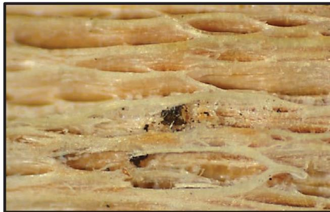
**Figure 4.1.** Specimen F, viewed under the stereomicroscope, showing weathered wood surface, open cellular structure, and weak cellular bonds. Note biological growth (center).
