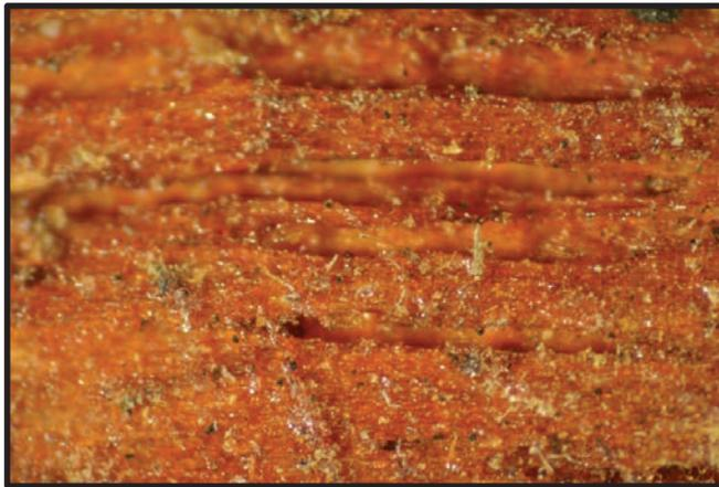
**Figure 4.4.** Specimen H showing remnants of a protective wood finish.
