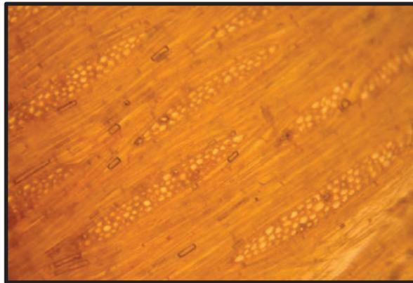
**Figure 4.15.** Tangential section of specimen H showing rays with 1 to 5 (but typically 3 to 4) cells in width at 100x magnification.
