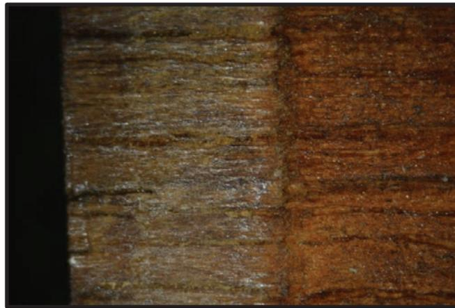
**Figure 5.12.** Specimen J showing the uncoated, protected top edge (left) and the surface treatment on the exposed face (right).
