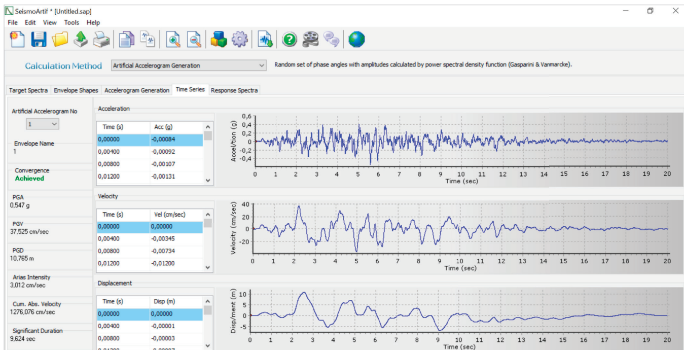
FIGURE 2.12. Example of an artificial spectrum-compatible generated accelerogram (SeismoArtif 2016 software, SeismoSoft).
