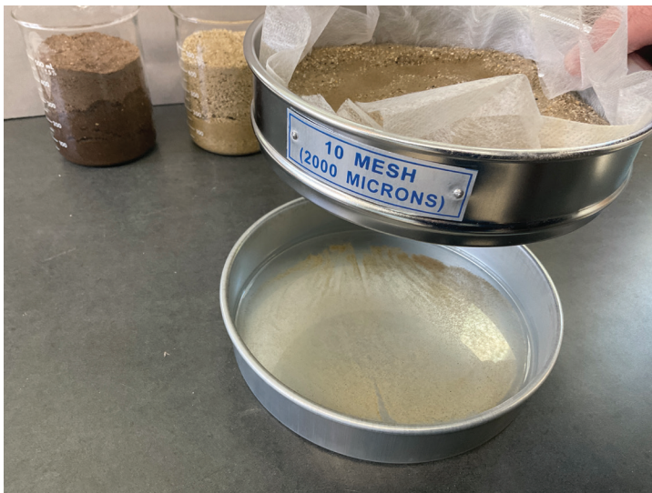
TEST 4 Water permeability test, evaluating a lightweight synthetic separation membrane, showing water and sand particles that have passed through the membrane.
