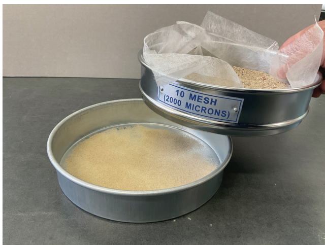
TEST 5 (DRY) Filtration test, showing the finest particles that have passed through the membrane (approx. 3x volume than that of wet test).
