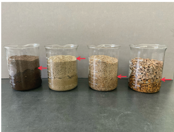
TEST 1 Example of different heights of capillary rise in soil, well-graded sand, large-grade sand, gravel. The well-graded sand shows best results for capillary water transport.
