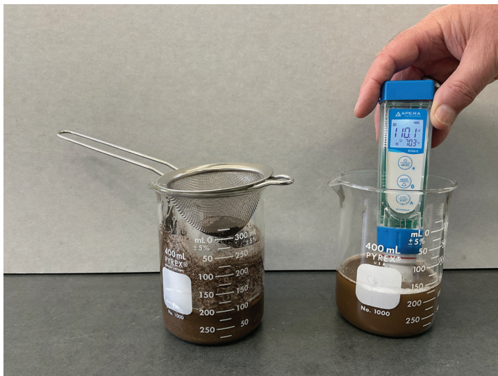
TEST 2 Measurement of conductivity of filtered liquid from a soil sample
