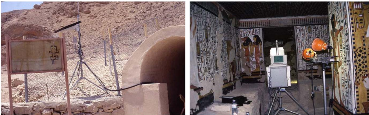
The environmental monitoring station installed at the tomb of Nefertari (QV 66) in August 1991. Left image shows a solar panel and sensors installed on a tripod just outside the entrance arch. Right image shows station's datalogger in the burial chamber.
