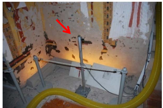
In addition to repairs noted above, a sensor to measure RH and T was installed in Chamber K (left) and an automated visitor counter was installed at the entrance to Chamber C (right).
