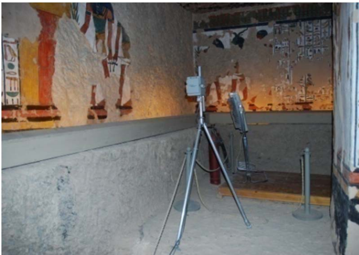
In addition to repairs noted above, a sensor to measure RH and T was installed in Chamber K (left) and an automated visitor counter was installed at the entrance to Chamber C (right).
