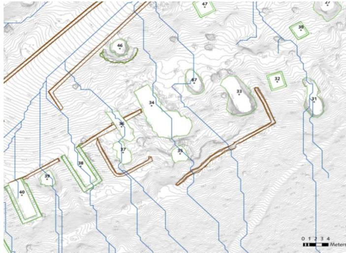
Part of the topographic map produced through laser scanning showing 10cm contour lines (gray), tomb openings (green), and drainage lines (blue) produced through ArcHydro software.
