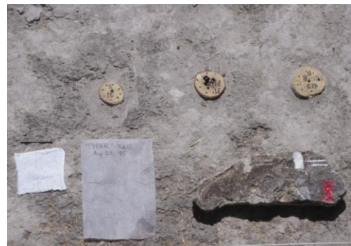
1995. Detail of indicator objects in trench (triangle carved in tuff, cotton fabric, geotextile, treated stumps and tuff block with various treatments).
