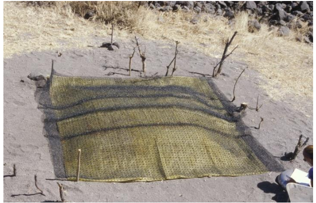
1995. Monitoring trench with Biobarrier 2 and Enkamat layers; acacia trees growing near the trench were pruned but not killed.
