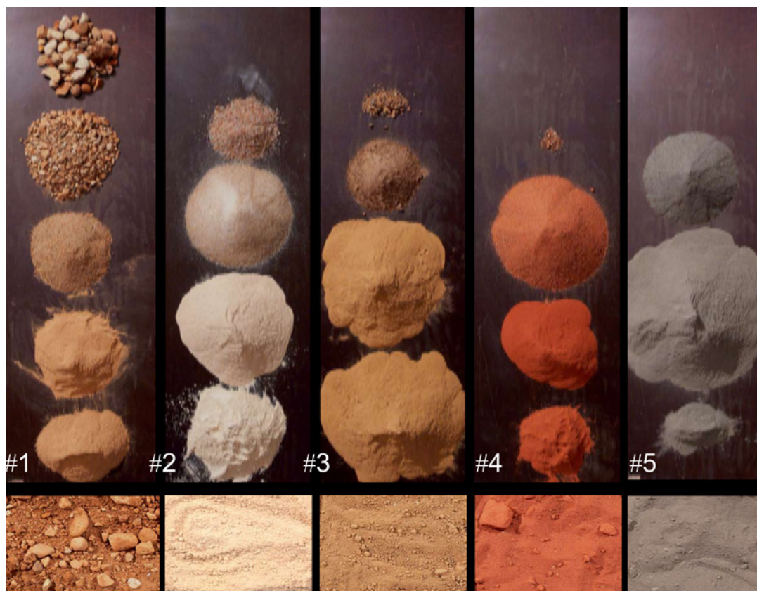
FIGURE 2.23. Five soil materials considered for earthen construction. Source: Laetitia Fontaine and Romain Anger. Soil #1 is a well-balanced mixture of stones, gravel, sand, silt, and clay, all present in roughly equal amounts. After compaction, it becomes a real, natural, very hard concrete containing enough clay to be highly cohesive and enough coarse grains to be rigid and avoid cracking. This earth is good for rammed-earth construction. Soil #2 contains many fewer stones and gravel. It is easier to work and to model by hand. Yet the amount of sand is large enough to avoid cracking when the material is used in the plastic state. This earth is ideal for making molded bricks. It is good for adobe construction. Soil #3 is very fine earth. It contains almost no stones and gravel, and the sand fraction is very small. It is very sticky when wet, but it cracks when it dries. Mixed with straw and/or sand to avoid cracking, this type of earth may be used as a filling material in a wooden frame. It is good for cob construction. Soil #4 contains neither stone nor gravel. It contains sand, silt, and clay in well-balanced amounts, but the clay fraction is smaller than in adobe earth, whereas the sand fraction is larger. This prevents cracking even when the material is mixed with a lot of water. This is an ideal material for coatings and mortars implemented in the viscous state. Soil #5 is very fine. It contains no stone, no gravel, no sand, and very little clay. The clay content is too small to impart some cohesion to the mixture. Using this material would lead to strength problems. Do not use it as it is.
