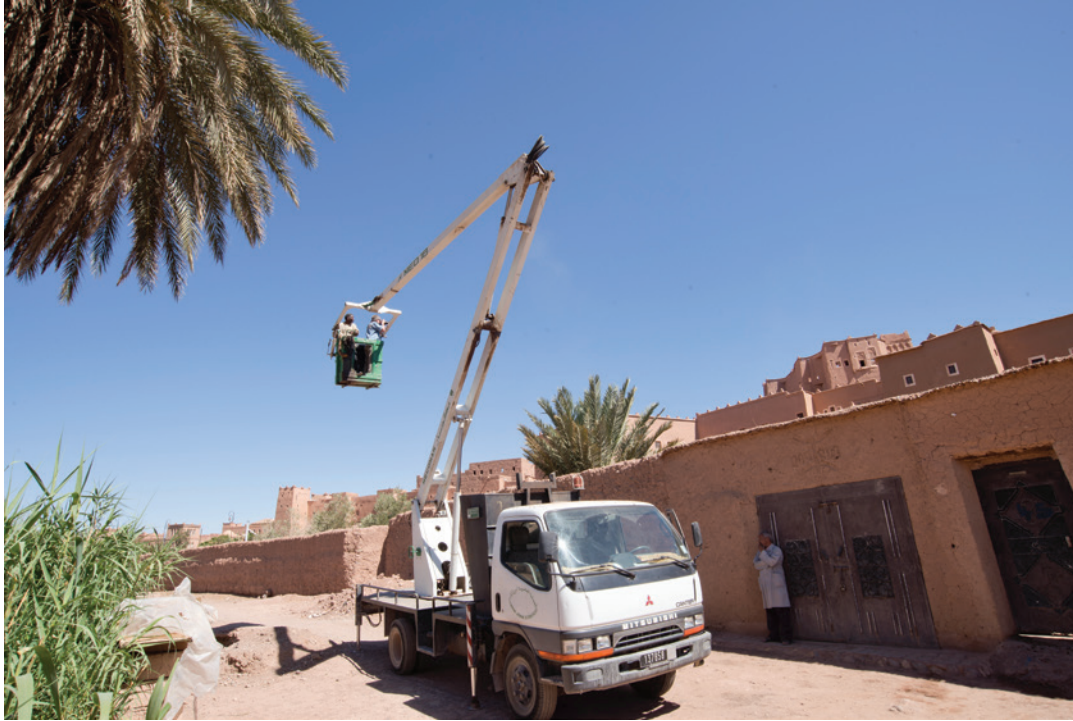
FIGURE 5.3. Technicians use an engineer's streetlight repair lift to photograph the site context for photogrammetric recording at the Kasbah of Taourirt, Ouarzazate, Morocco. Source: Mario Santana Quintero.
