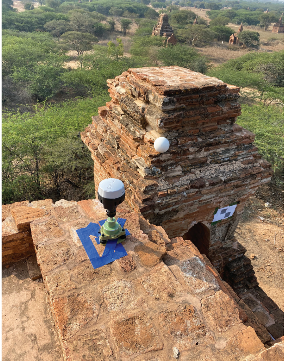
FIGURE 5.4. In site documentation, a GNSS device is used to record coordinates to georeference a survey network at the Tha-mu-ti-hpaya temple (Bagan World Heritage Site, Myanmar). Source: Mario Santana Quintero.
