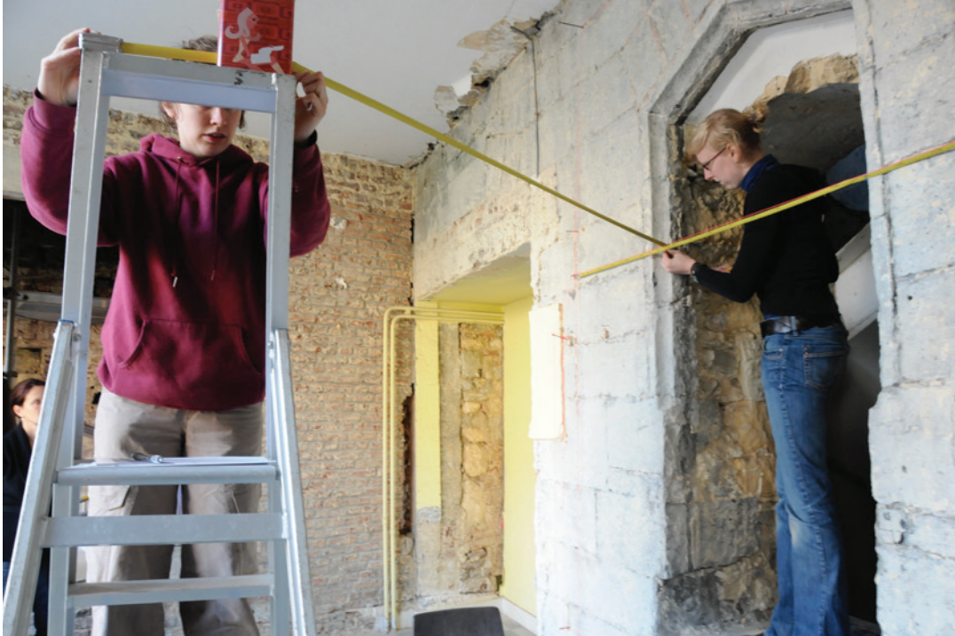
FIGURE 5.7. Technicians conduct a hand survey to prepare a field note using trilateration at a historic building in Liège, Belgium. Source: Mario Santana Quintero.
