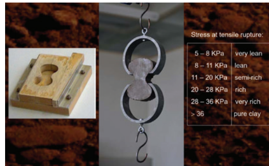
FIGURE 2.15. The wet cohesive strength test of soils and the mold used to shape the specimen. Source: Schroeder (2016) and ZRS, Christof Ziegert.
