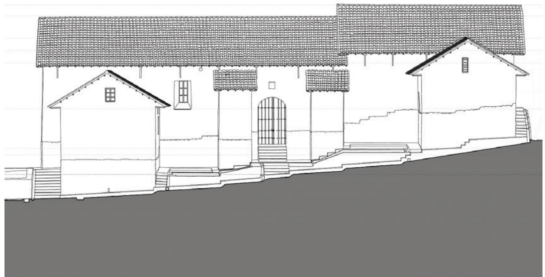
FIGURE 5.18. A measured drawing of the north elevation of the church of Kuñotambo, Peru. This record has been produced with the total station survey, aerial photography, and photogrammetry to produce an ortho-corrected image, which has been traced using CAD. Source: Miquel Reina Ortiz and Mario Santana Quintero, Carleton Immersive Media Studio.
