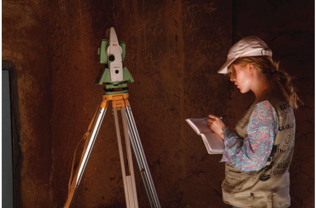
FIGURE 5.8. A technician conducts a total station measurement in the interior of the Kasbah of Taourirt, Morocco. Source: Mario Santana Quintero.
