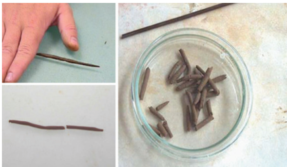
FIGURE 2.13. The PL is determined by remolding a small ball of moist plastic earth and manually rolling it out into a 3 mm thread (min. length: 5 cm). The PL is the moisture content at which the thread crumbles into 1 to 2 cm pieces before being completely rolled out (ASTM D4318). Source: Schroeder (2016).
