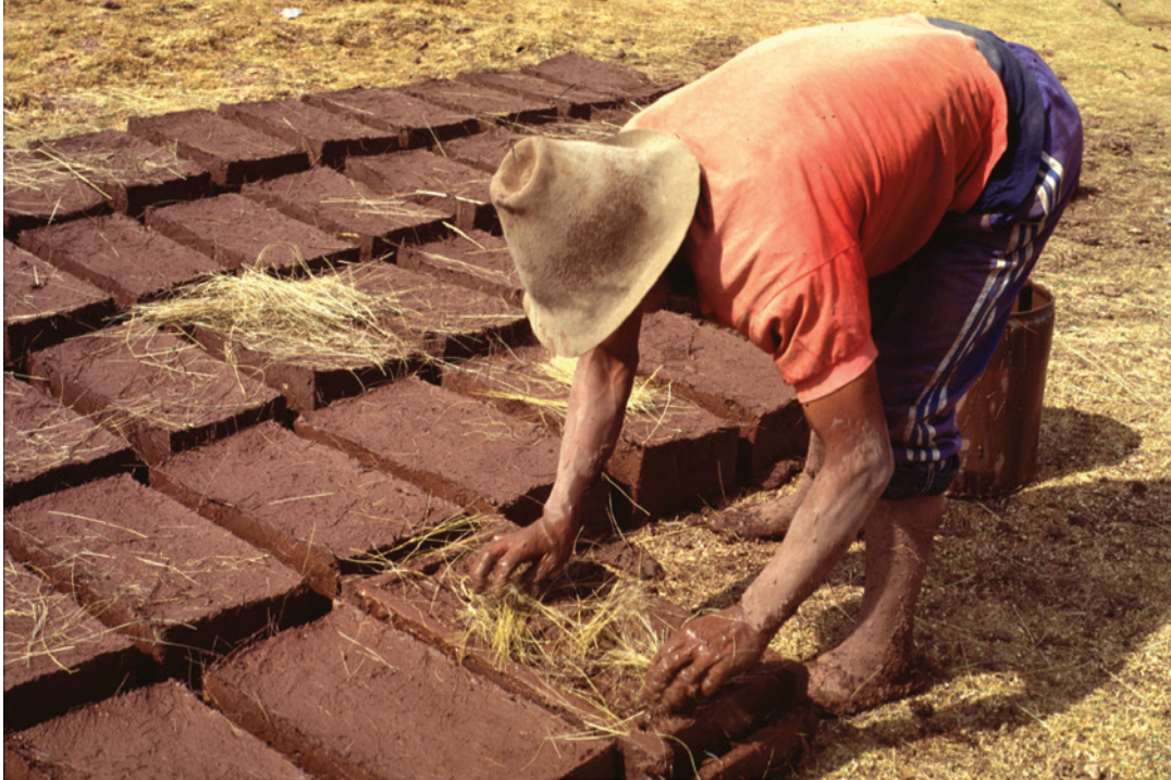
FIGURE 3.8. Individual artisan production of adobe. Source: Wilfredo Carazas Aedo.
