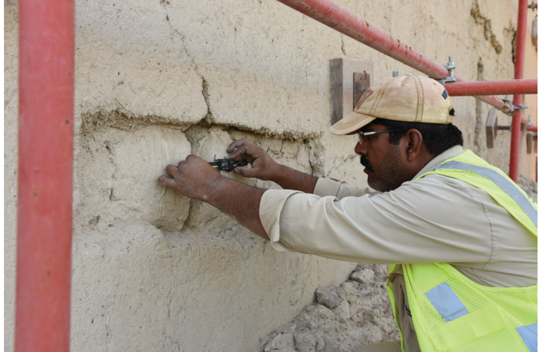
FIGURE 11.6. Monitoring cracks at Muraijeb Fort, Al Ain. Source: DCT Abu Dhabi.
