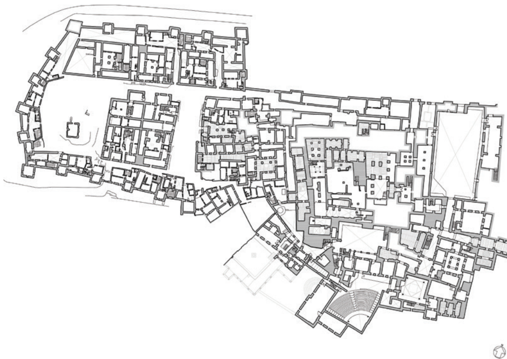
FIGURE 5.13. A measured line drawing of the floor plan of the Kasbah of Taourirt, Morocco. This record has been produced with total station survey, photogrammetry, and CAD. Source: Carleton Immersive Media Studio.
