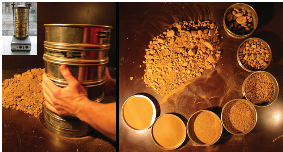
FIGURE 2.4. Sieve set used for the particle-size analysis of the coarse fraction of soils (gravel and sand). After sieving, the mass of material retained on each sieve is weighed, and the cumulative passing percentage is calculated. Source: Fontaine and Anger (2009). The inset shows a sieve set on a mechanical shaker. Source: Schroeder (2016).
