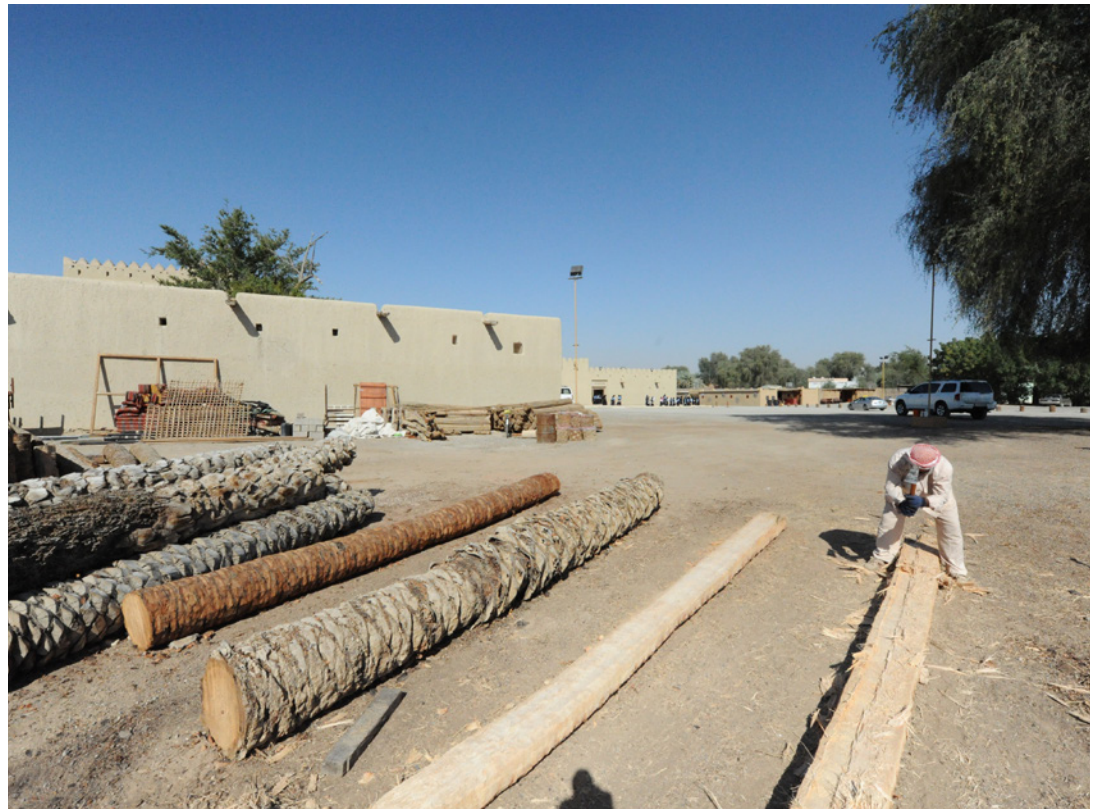
FIGURE 7.34. Traditional method of preparing palm beams at the DCT workshop: palm trunks are usually sourced from old trees, dried over a period of three to six months, cut down to size, and stored until needed. Source: DCT Abu Dhabi.
