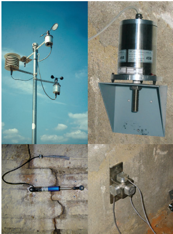
Clockwise from top left: weather station; biaxial inclinometer, which measures tilt in both north–south and east–west directions; accelerometers, which measure three-axis seismic acceleration; transducers, which measure strain on cracks. Photos: © Giorgio Croci.
