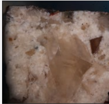
Upper stratigraphy of BCN_58 (upper west wall, south side) showing the clear absence of a pink-tinted plaster layer.
