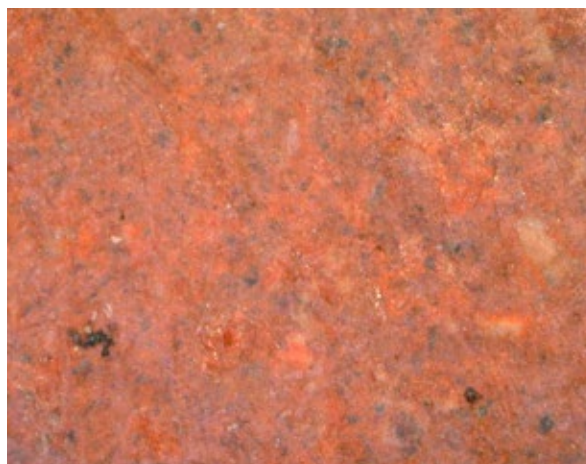
FIGURE 5.17 Micrograph showing flecks of carbon black present throughout the red monochrome background paint mixture.
