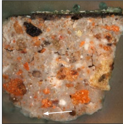
Cross section of BCN_42 (lower south wall, west side) showing the unique plaster found with the brick dust as aggregate. Layer 2 is indicated by the white arrow.
