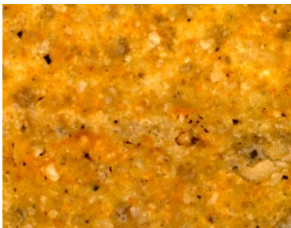
FIGURE 5.16 Micrograph showing flecks of carbon black present throughout the yellow monochrome background paint mixture.
