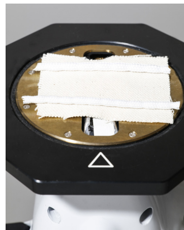
FIGURE A2.2. Use of weighted ropes to flatten the paint mock-up on top of the XRF stage and head. Here, the painted surface is directly facing the XRF aperture. Ropes should be kept away from the aperture so as not to contribute to spectral response.
