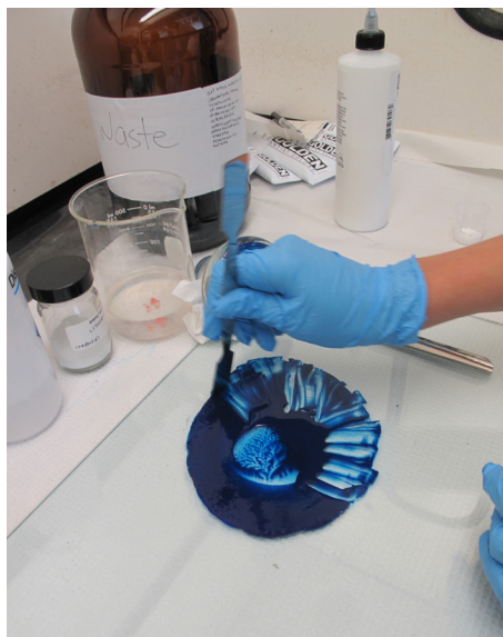
FIGURE A2.13. Paint being scraped toward the middle of the glass sheet before transferring to a jar.
