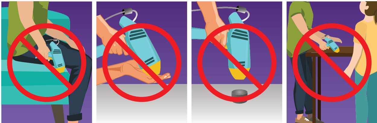
FIGURE 1.5. Illustrations of spectrometer handling that risk exposure to radiation. From left: holding the instrument too close to the body; holding the sample in the hand; holding the nose of the instrument too far away from the sample; having another person in the scattering angle of the radiation.
