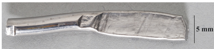
FIGURE 3.6. Flattened lead-tin solder. Use of a rubber mallet has created lines on the side of impact. The other side is smoother, with no lines; that side should be used in exercise 3.1f.
