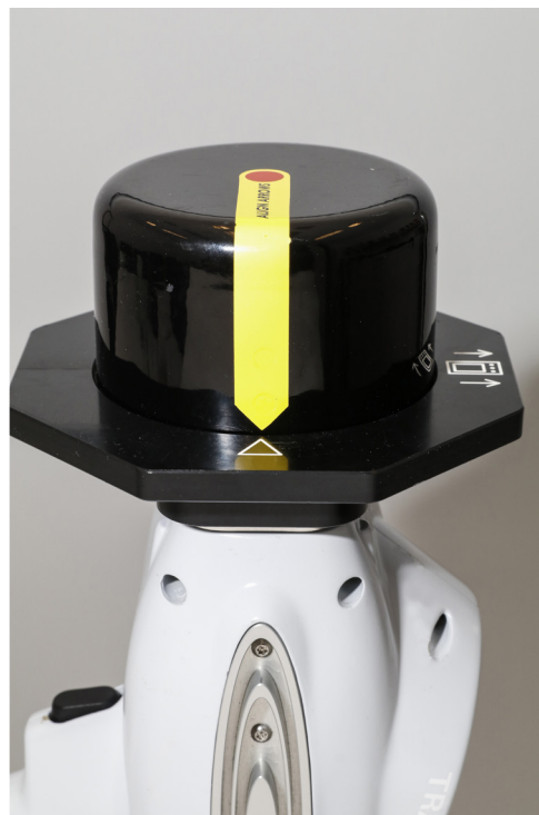
FIGURE 1.6. Photo of the Bruker Tracer III-SD, showing a safety cap placed over the sample to be analyzed, to minimize risk of exposure.
