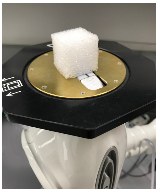
FIGURE 2.18b. Polyethylene foam cube sample sized to fit underneath the cap and fully cover the aperture.
