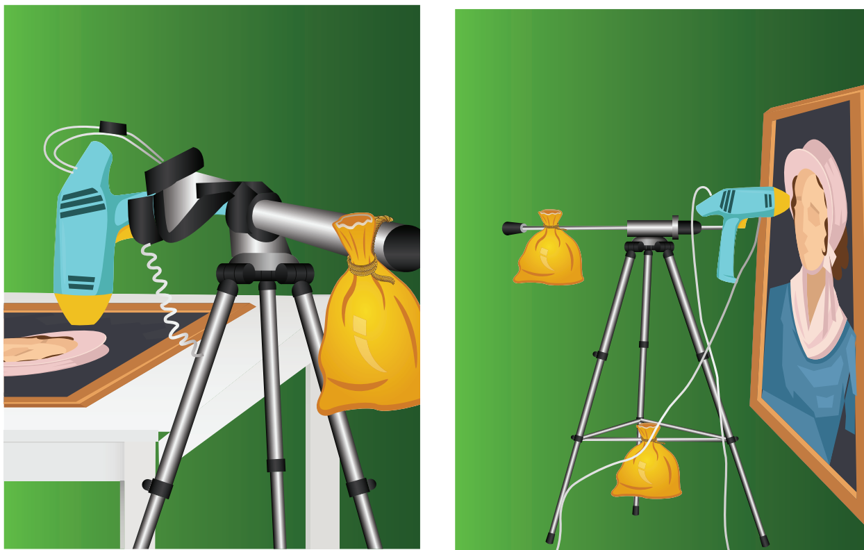
FIGURE 4.4. XRF instrument tripod setup with counterweights for an object mounted horizontally (left) and vertically (right).
