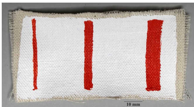
FIGURE A2.4. Photo of mock-up: cadmium red lines of varying widths painted on top of a titanium white underlayer on top of bare canvas.
