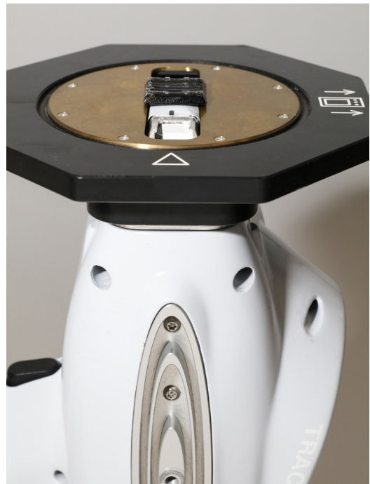
FIGURE 3.4. Photo showing the glass sample, smooth side facing the XRF nose on the Bruker III-SD unit head. (See chap. 1, fig. 1.6 for use of the safety cap.)
