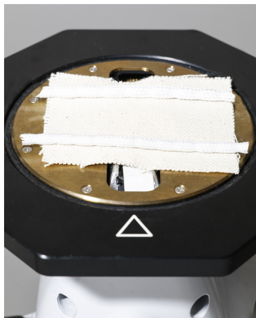
FIGURE 3.5. Photo showing position of the sample on the XRF head, with weights to ensure the canvas lies flat. Painted surface is directly facing the XRF aperture.
