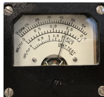
FIGURE 1.8c. Display on the Ludlum Model 3, showing cpm, milliRoentgen per hour (mR/hr) measured.
