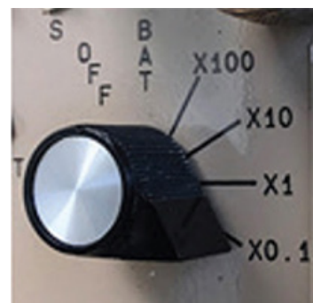
FIGURE 1.8b. Range selector switch on the Ludlum Model 3 survey meter.
