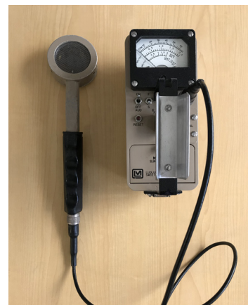
FIGURE 1.8a. A Geiger-Muller pancake detector attached to a Ludlum Model 3 portable survey meter (count rate indicator).
