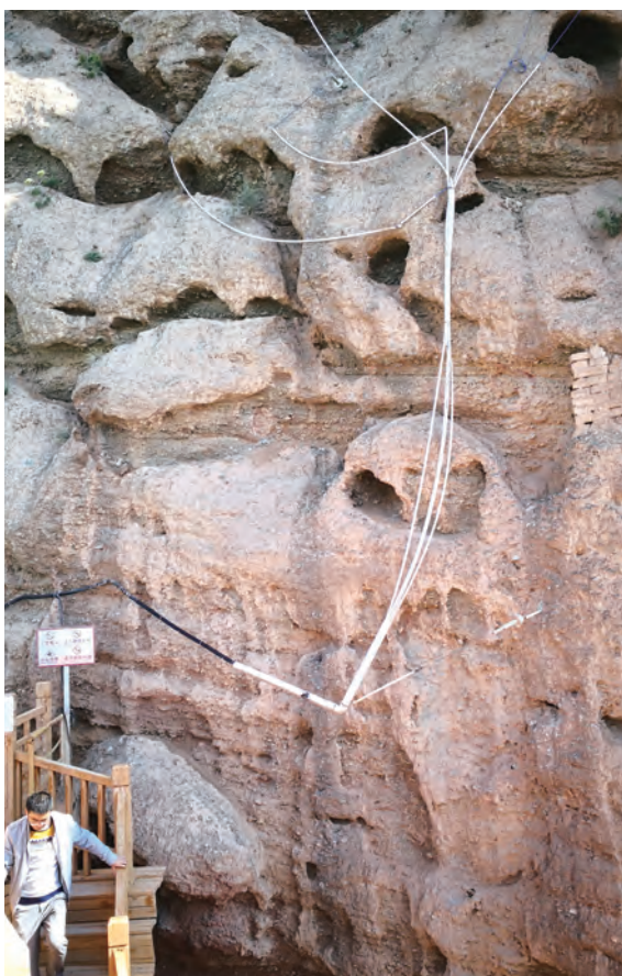
Wiring from monitoring instruments should be minimized or hidden as much as possible, not exposed to view as here.
